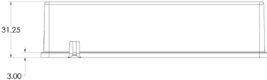
Figure A-6 Reagent Plate Side View Dimensions
