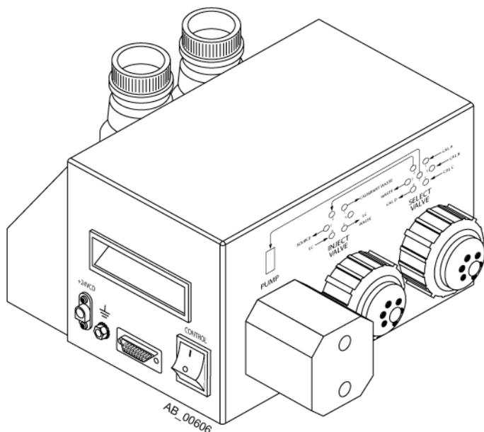
The CDS is a separate component installed on top of the mass spectrometer. It connects to the gas and vacuum bulkhead on the left side of the mass spectrometer with a Control cable.
