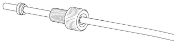
2. Insert the tubing into the pump as far as it will go, to prevent dead volumes from appearing in the clear FEP tubing, and then tighten the nut.
