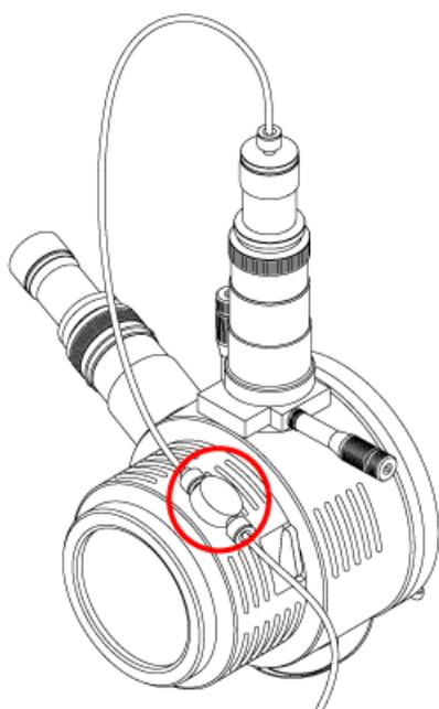
3. Connect a 30 cm piece of red PEEK tubing to the grounding union.
