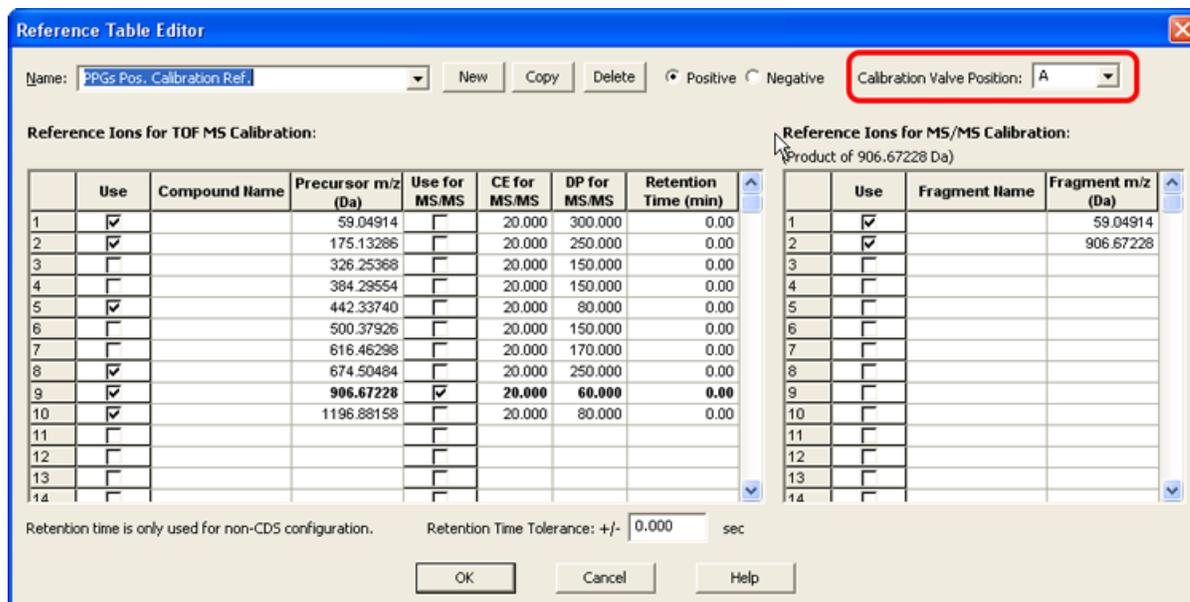
4. In the **Calibrant Valve Position** field, select the calibrant valve: Cal B (valve 6), Cal C (valve 5), or Cal D (valve 4).
