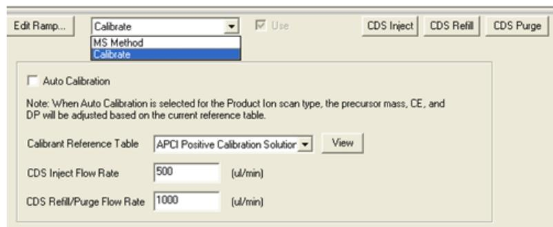
6. In the **Calibrant Reference Table** field, select the required calibrant reference table.
