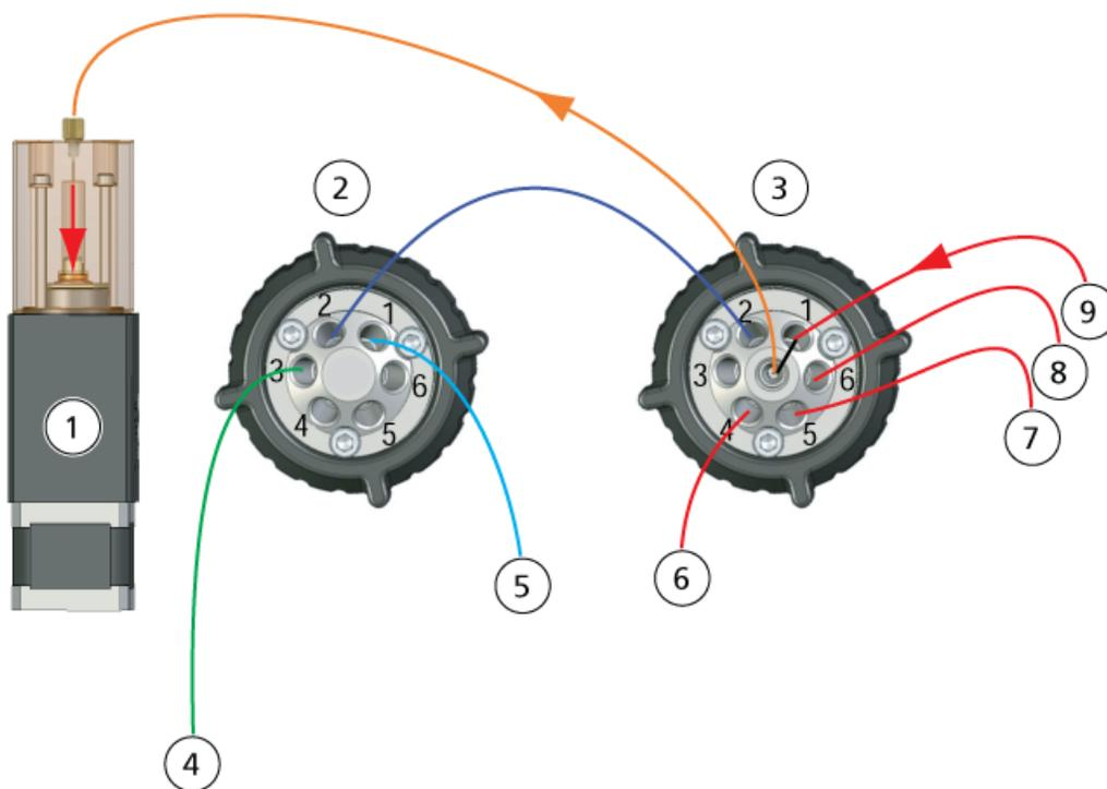
Figure 1-5 Purge Mode, Inject Cycle
