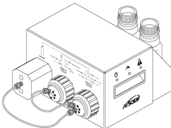
6. For the calibrant line, assemble the ferrule and Rheodyne fitting on the 60 cm clear FEP tubing, insert the tubing into the Select valve CAL A port as far as it will go, and then tighten the fitting.
