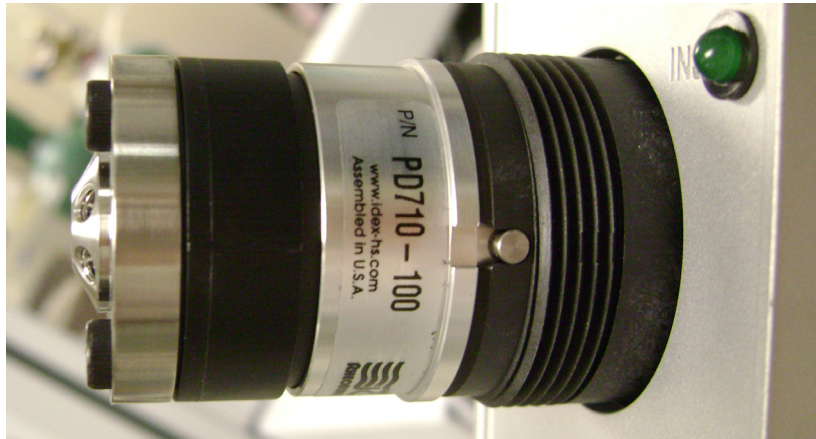
Figure 4-10 Valve Pod—Side View, Showing Pin in Notch
