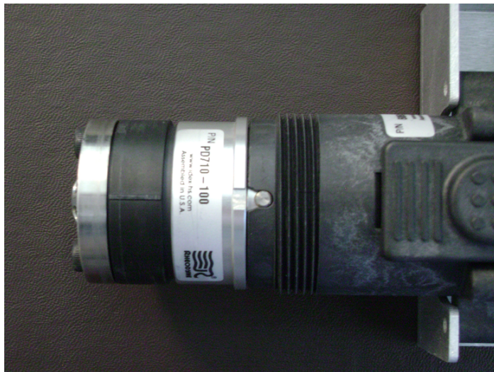
Figure 7-14 Valve Pod–Side View, Showing Pin in Notch
