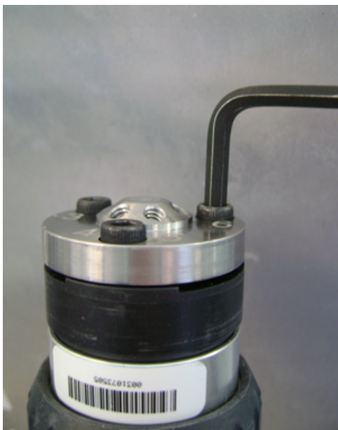
Figure 7-11 Unscrewing the Valve Stator
