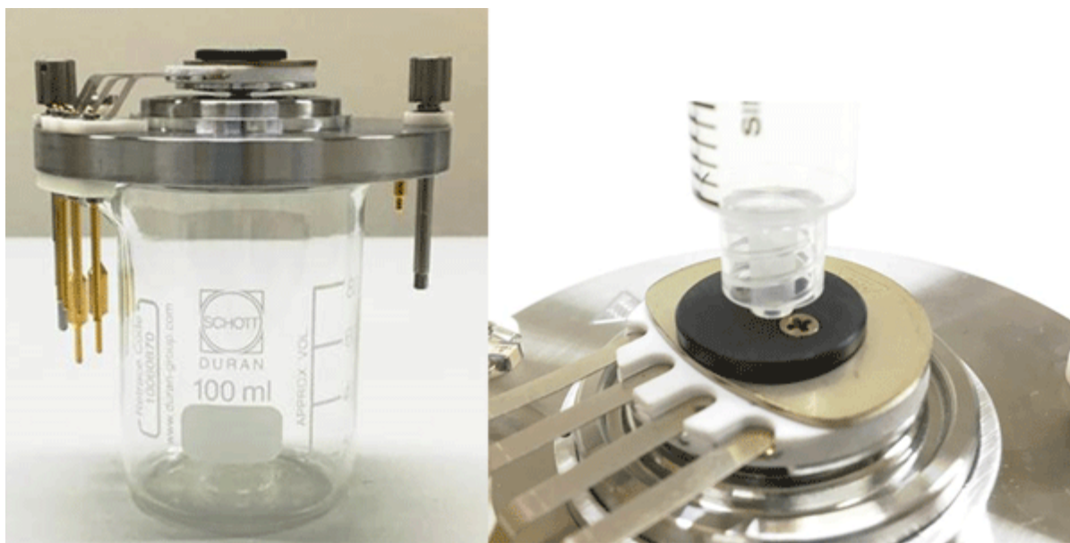
Figure 4-6 Nano Cell Heater Assembly on the Beaker and Syringe
