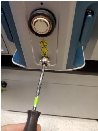
Figure 3-4 Tighten the Screw
