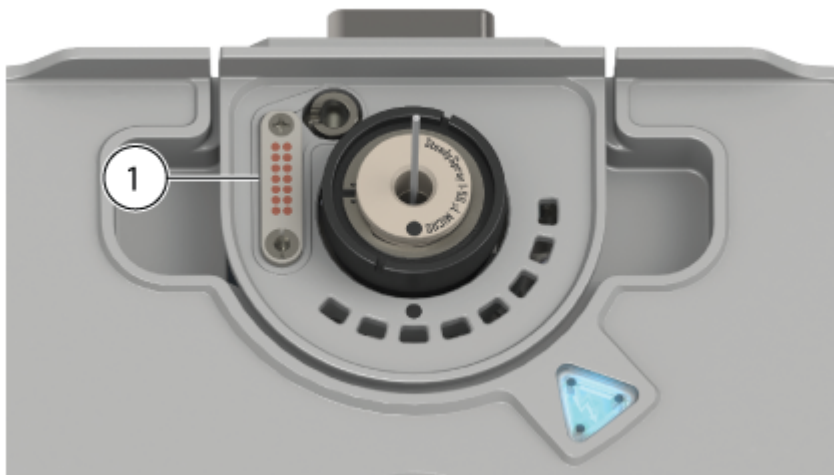
Figure 4-2 Contact Pad on ESI Module
