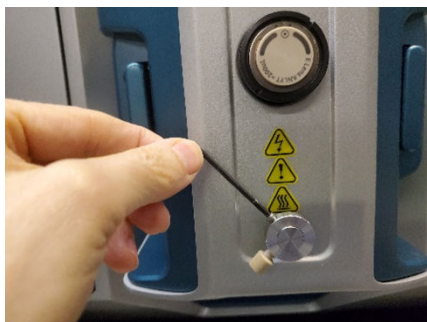
Figure 3-7 Tighten the Captive Screw
