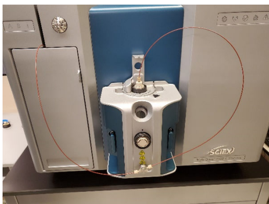
Figure 3-8 PEEK Tubing Connected
