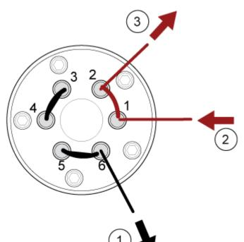
Figure 3-4 Diverter Valve—Diverter Mode Position A
