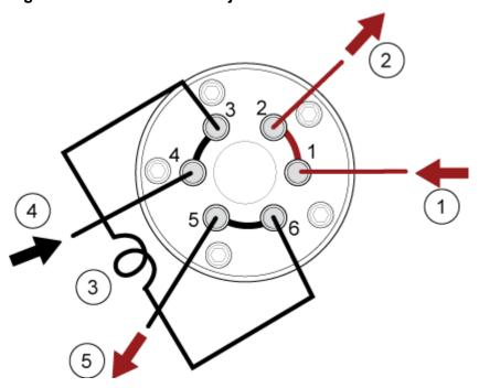
Figure 3-3 Diverter Valve—Injector Mode Position B
