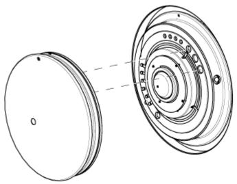
The curtain plate is held in place by three retaining ball catches mounted on the orifice plate.
