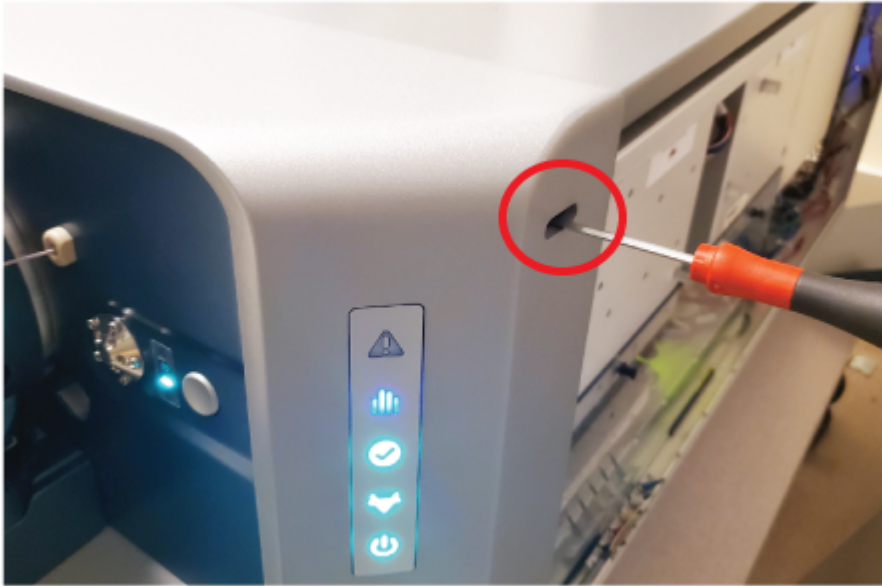
Figure 5-17 Hole in Front Dress Panel
