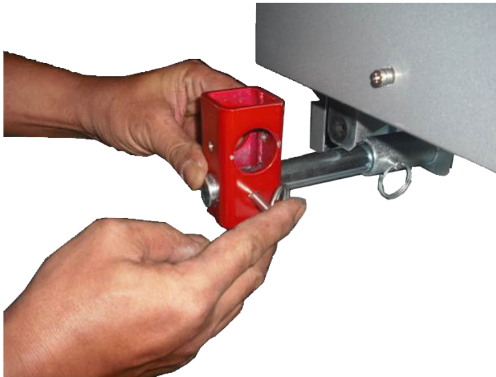
Figure 5-10 Short Block Installed
