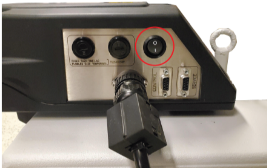
Figure 3-1 Oil-Sealed Roughing Pump: On/Off Switch
