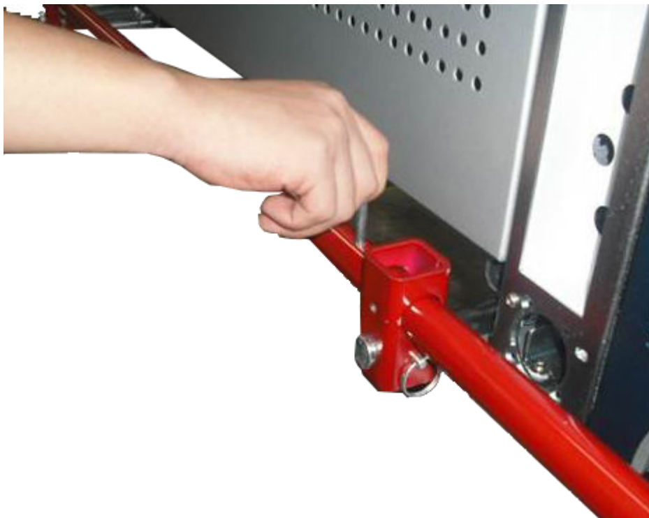
Figure 5-11 Installing the Locking Pin on the Log Rod
