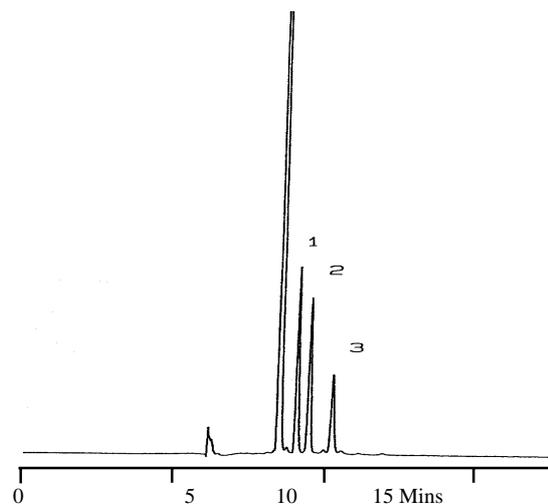
**Figure 7.**  $3\mu\text{m}$  Spherisorb ODS-1 40cm packed, 55cm total length, Mobile phase: 90% Acetonitrile / 10% 0.1M Tris, Detection at 238nm, Applied voltage: 30kV, Temperature 30°C, Injection: 10 kV/30 seconds, Peak identity: A=Fluticasone propionate 1=closely related impurity 2=Des flouro analogue 3=hydrophobic impurity. Reproduced by permission of publishers, reference 35.
