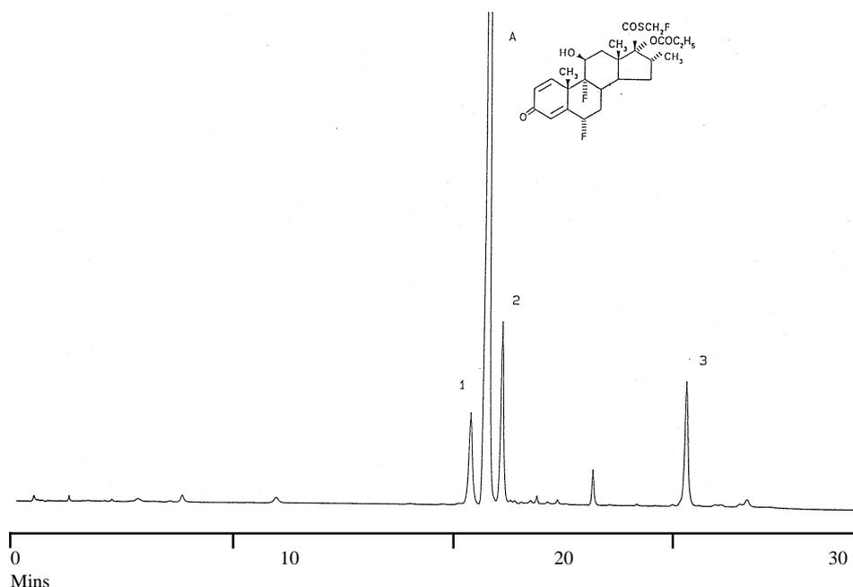
**Figure 5.**  $3\mu\text{m}$  Spherisorb ODS-1 15cm x 4.6mm i.d., Gradient: 40% Acetonitrile/ $\text{H}_2\text{O}$  to 70% Acetonitrile/ $\text{H}_2\text{O}$  in 20 minutes (EXP 5), Detection at 238nm, Flow: 1.0ml/min, Peak Identity: A=Fluticasone propionate 1=closely related impurity 2=Des fluoro analogue 3=hydrophobic impurity. Reproduced by permission of N.W. Smith.
