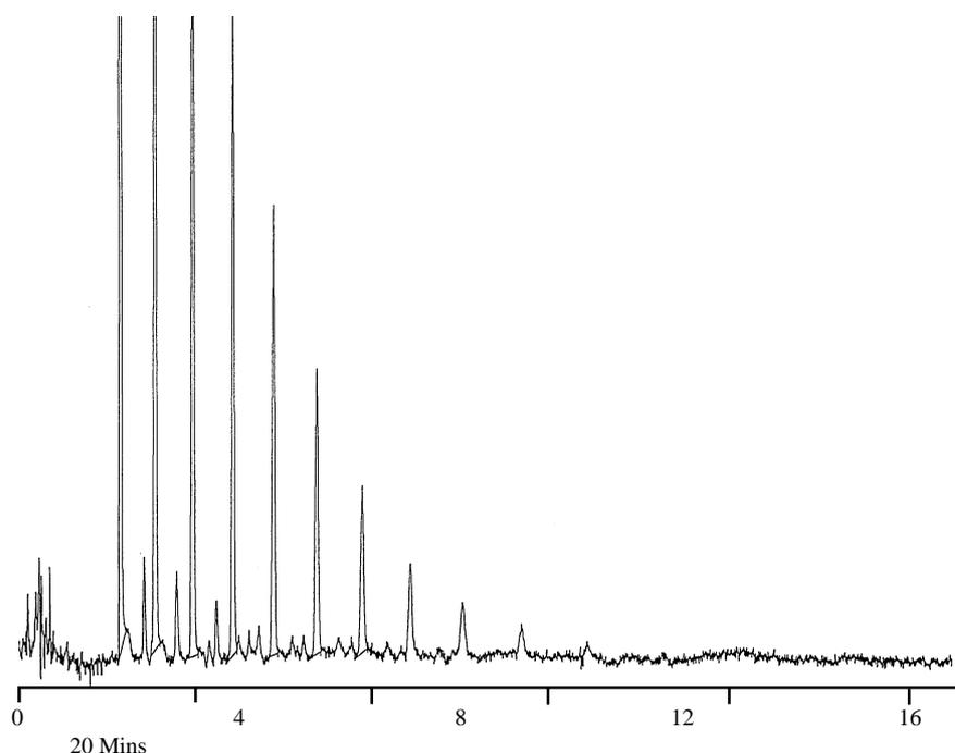
**Figure 12.**  $3\mu\text{m}$  Spherisorb SCX , Mobile phase: 70% Acetonitrile / (30% 0.05M  $\text{NaH}_2\text{PO}_4$  pH2.3), Detection at 254 nm, Applied voltage: -30kV, Temperature  $30^\circ\text{C}$ , Injection: -5kV/5secs. Reproduced by permission of N.W. Smith.
