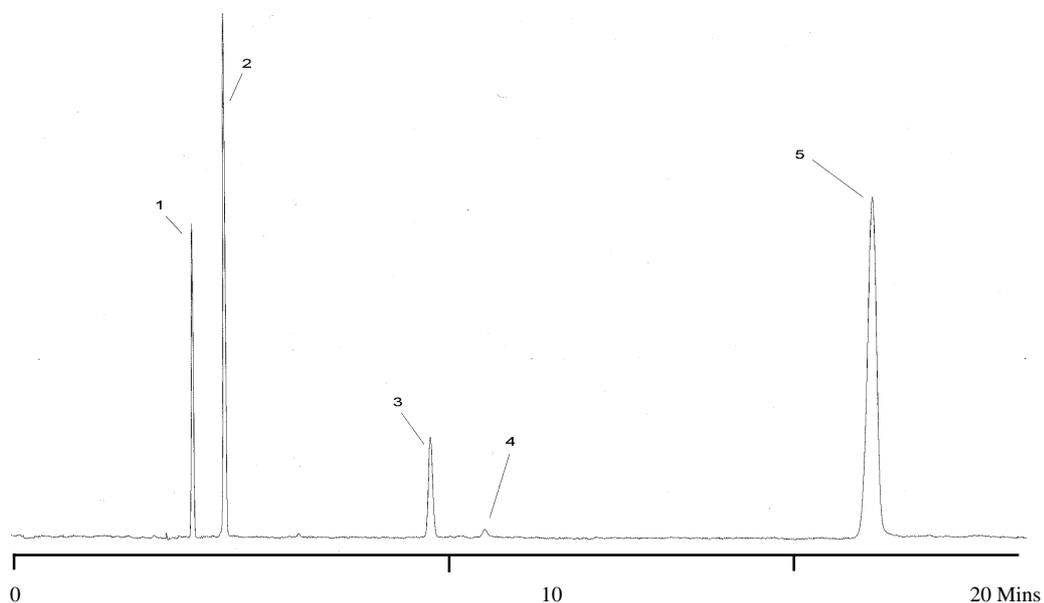
**Figure 2.**  $3\mu\text{m}$  Spherisorb ODS-1, Mobile phase: 70% Acetonitrile / 30 (20mM  $\text{NaH}_2\text{PO}_4$  pH 2.3), Detection 210nm, Applied voltage: 30kV, Temperature  $30^\circ\text{C}$ , Injection: 5kV/10 seconds, Peak identity: 1= Thiourea 2=GR57888X 3=Fluticasone propionate 4=Des flouro analogue 5=GR57794X. Reproduced by permission of N.W. Smith.
