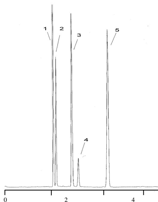
**Figure 1.**  $3\mu\text{m}$  Spherisorb ODS-1, Mobile phase: 70% Acetonitrile / 30% 0.01M  $\text{Na}_2\text{HPO}_4$ , Detection 210 nm, Applied voltage: 30kV, Temperature  $30^\circ\text{C}$ , Injection: 10kV/5 seconds, Peak identity: 1= Thiourea 2=GR57888X 3=Fluticasone propionate 4=Des flouro analogue 5=GR57794X. Reproduced by permission of N.W. Smith.
