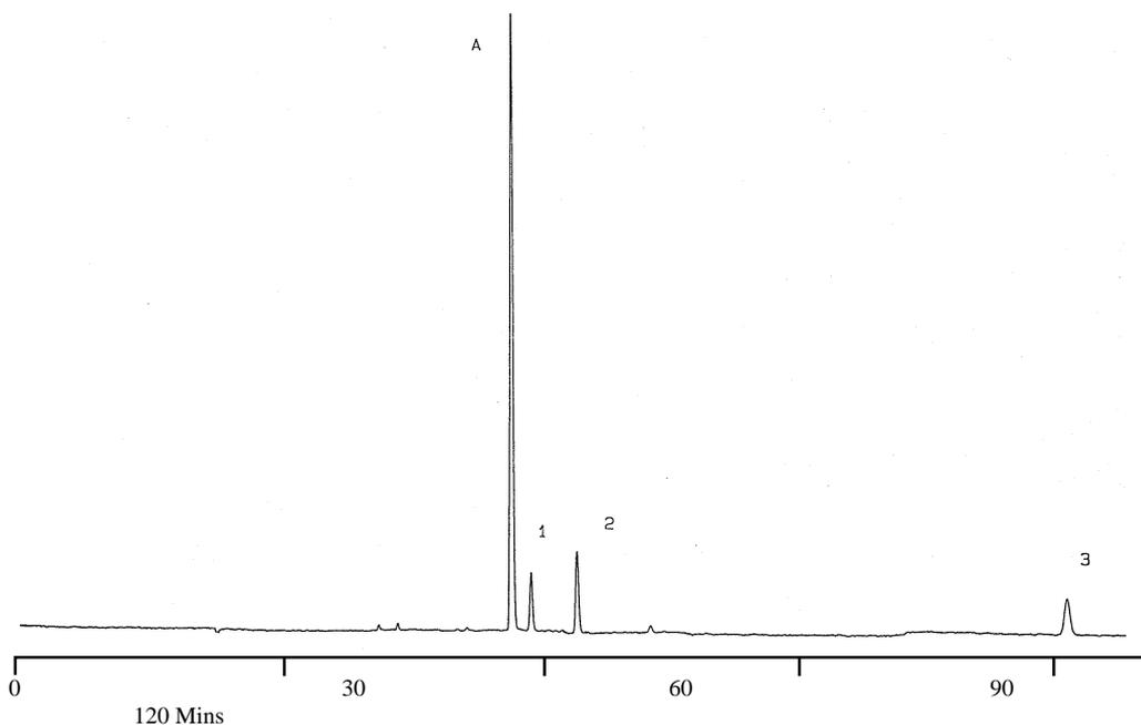
**Figure 6.**  $3\mu\text{m}$  Spherisorb ODS-1 40cm packed, 55cm total length, Mobile phase: 75% Acetonitrile /  $\text{H}_2\text{O}$  + 2mM  $\text{Na}_2\text{HPO}_4$ , Detection at 238nm, Applied voltage: 30kV, Temperature  $30^\circ\text{C}$ , Injection: 20 kV/10 seconds, Peak identity: A=fluticasone propionate 1=closely related impurity 2=Des flouro analogue 3=hydrophobic impurity. Reproduced by permission of publishers, reference 9.
