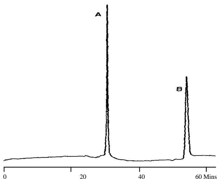
**Figure 13.** Partisil-10-ODS-2 (170 $\mu$ m i.d. capillary) Packed length 58cm, Applied voltage: 30kV, Peak A=9-methylanthracene B=perylene. Reprinted from *Journal of Chromatography*, 218 (J.W. Jorgenson and K.D. Lukacs) *High-Resolution Separations based on Electrophoresis and Electroosmosis*, 209-216 (1981) with kind permission of Elsevier Science-NL, Sara Burgerhartsraat 25, 1055 KV Amsterdam, The Netherlands.
