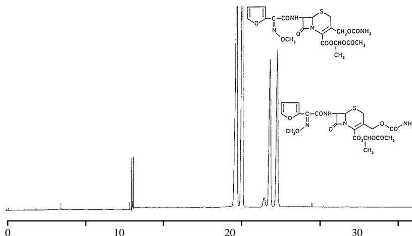
**Figure 10.** 3 $\mu$ m Spherisorb ODS-1 40cm packed, 55cm total length, Mobile phase: 50% Acetonitrile / 50% 0.01M Na<sub>2</sub>HPO<sub>4</sub>, Applied voltage: 30kV, Temperature 30<sup>o</sup>C, Injection: 20kV/0.2min. Reproduced by permission of the publishers, Ref. 9.
