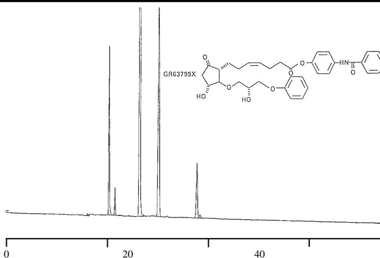
**Figure 11.** 3 $\mu$ m Spherisorb ODS-1 60cm packed, 82cm total length, Mobile phase: 70% Acetonitrile / 30% 0.01M Na<sub>2</sub>HPO<sub>4</sub>, Applied voltage: 30kV, Temperature 35<sup>o</sup>C, Injection: 30kV/0.4 min. Reproduced by permission of N.W. Smith.
