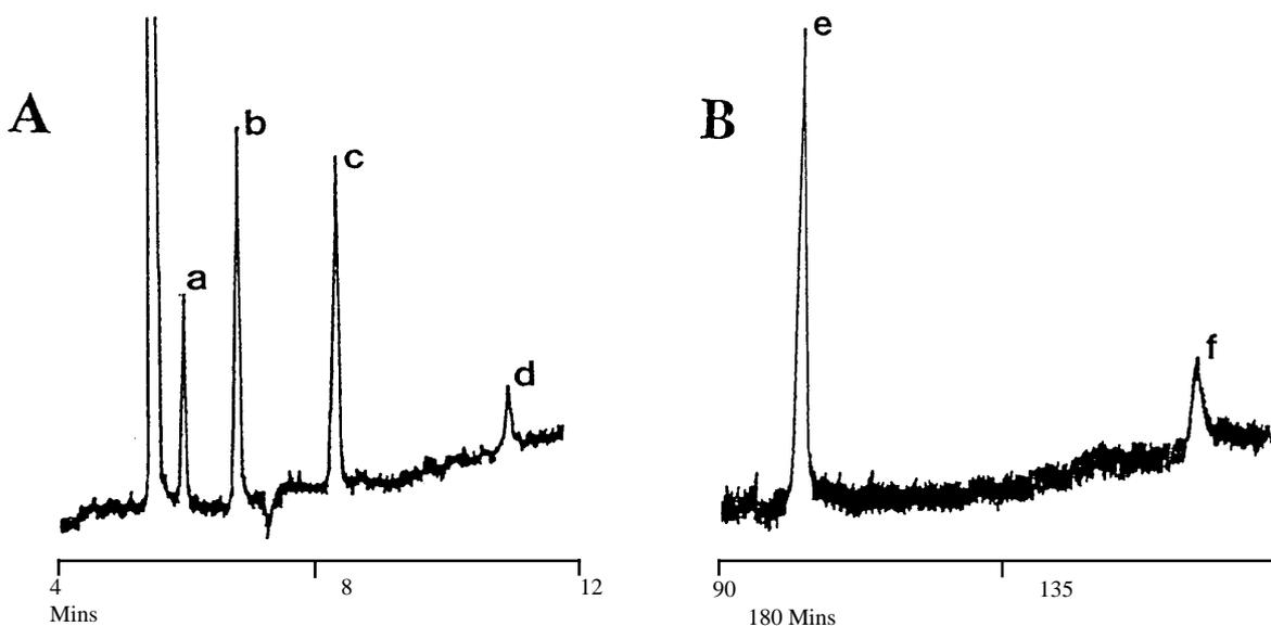
**Figure 14A / 14B.** Electropherogram A, Peak Identities: a)Benzene, b)Anthracene, c)BaP, d)Coronene, 80/20 Acetonitrile/Methylene Chloride, Applied Voltage 20kV. Electropherogram B, Peak Identities: e)C<sub>60</sub>, f) C<sub>70</sub>, 50/50, Acetonitrile/THF, Applied Voltage 20kV. Reproduced by permission of publishers, reference 23.
