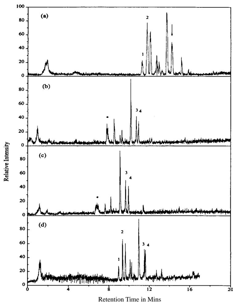
**Figure 9.** Separation of Bovine cytochrome *c* digest using a 20min, 0-50% acetonitrile gradient with 8pmole sample injections, column length 6.0cms. Operating conditions: a)HPLC mode with a back pressure of 90 bar; b)1000V applied voltage with 50 bar pressure; c)1400V applied voltage with 50 bar pressure; d)600V applied voltage with 70 bar pressure. Reproduced by permission of publishers, reference 14.
