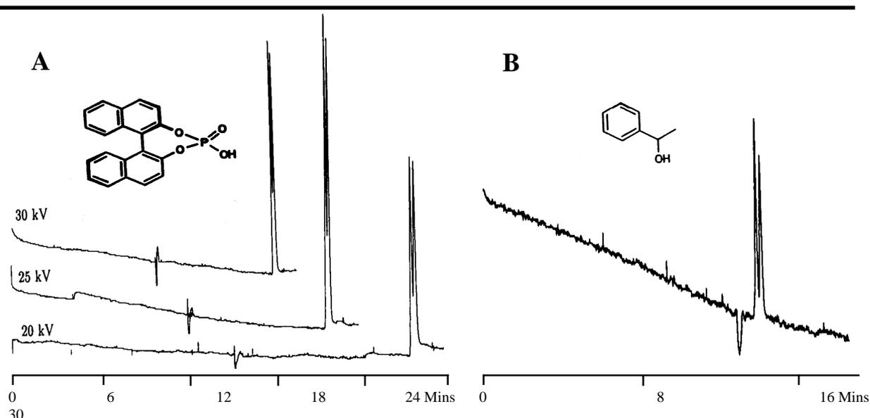
**Figure 15.** Chirasil-Dex (50  $\mu\text{m}$  I.D. capillary) Effective length 80cms, Borate-phosphate buffer, pH=7, Detection at 220nm, Temperature 20°C buffer. Electropherogram A=Applied voltages, 20,25,30kV and B=Applied Voltage of 20kV. Reproduced by permission of S. Mayer and V. Schurig, *J. High Resol. Chromatogr.*, 15,129-131 (1992).
