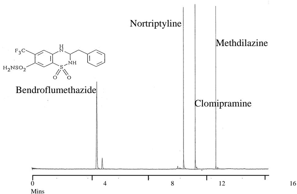
**Figure 18.**  $3\mu\text{m}$  Spherisorb SCX, Mobile phase: 70% Acetonitrile / 30% (0.05M  $\text{NaH}_2\text{PO}_4$  pH 2.3), Applied voltage: 30kV, Temperature  $30^\circ\text{C}$ , Injection: 2kV/0.5min, Detection at 220nm. Reproduced by permission of publishers, Ref. 35.
