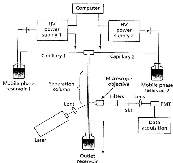
*Schematic of the solvent gradient elution CEC apparatus. Reproduced by permission of publishers, reference 13. First published in LC-GC International, Vol. 10, Number 3 (1997).*
