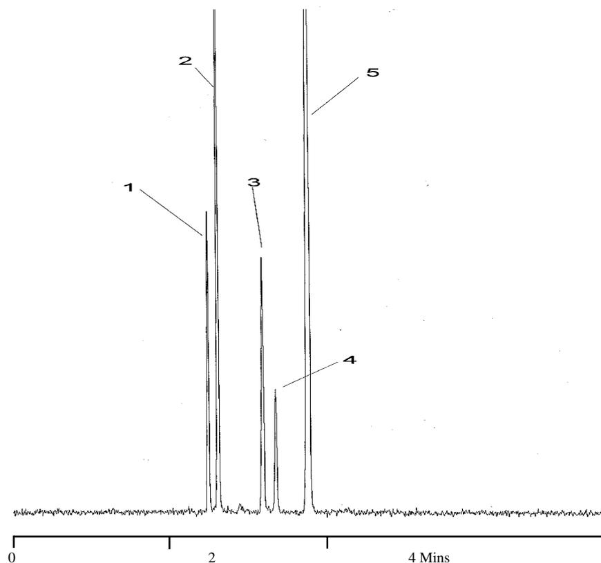
**Figure 4.**  $3\mu\text{m}$  Spherisorb C<sub>6</sub>/SCX, Mobile phase: 70% Acetonitrile / (30% 0.05M NaH<sub>2</sub>PO<sub>4</sub> pH 3.5), Detection at 210 nm, Applied voltage: 30kV Temperature 30°C, Injection: 10kV/5 seconds, Peak identity: 1= Thiourea 2=GR57888X 3=Fluticasone propionate 4=Des flouro analogue 5=GR57794X. Reproduced by permission of N.W. Smith.
