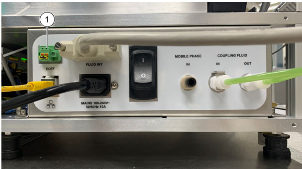
Figure 6-3 Emergency Off Connector and Plug on the Back Panel of the Echo ® MS Module
