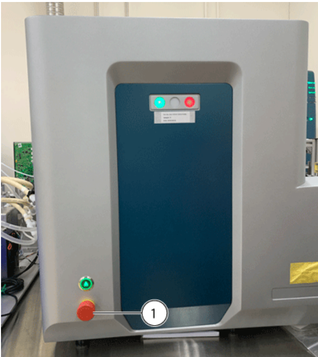
Figure 6-2 Emergency Off Button on the Front Panel of the Echo ® MS Module
