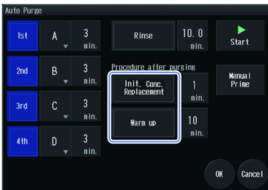
Figure 5-10 Init. Conc. Replacement and Warm Up
