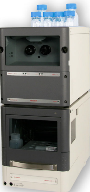
Figure 3-7 Eksigent NanoLC Ultra with NanoLC AS-2 autosampler
