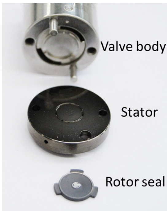
Figure D-7 Six-port Valve Components
