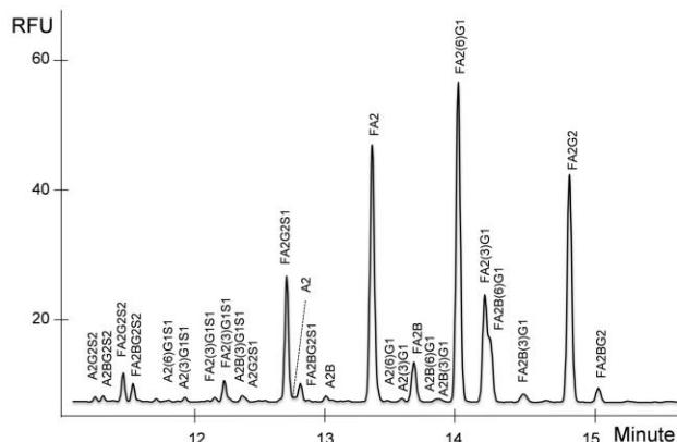
**Figure 1.** CE-LIF trace of IgG N-glycan structures from human serum. Conditions: 50 cm effective length (60 cm total) N-CHO coated, 50  $\mu$ m i.d. capillary columns filled with N-CHO Carbohydrate Separation Gel Buffer, E=500 V/cm, reversed polarity, Samples were injected by pressure: 1 psi (6.89 kPa) for 5 sec.
