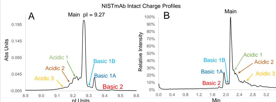
Figure 2. A is a UV 280 nm absorbance image of NISTmAb charge isoform peaks separated by icIEF. Figure 2 B is the base peak electropherogram (BPE) of same corresponding peaks after mobilization, electrospray and analysis by MS. The UV and BPE profiles are mirror images of each other as charge variants with higher pI are the first to be analyzed in the MS.
