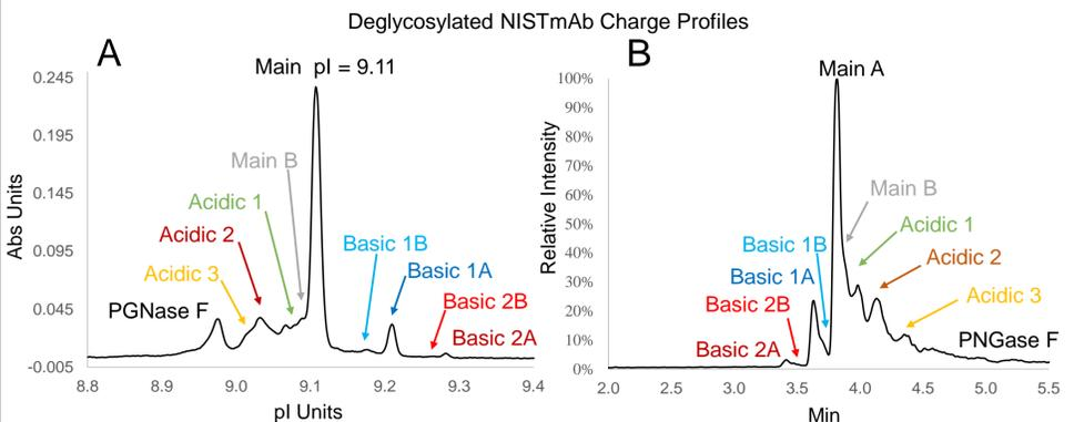
Figure 3 A is a UV 280 nm absorbance image of deglycosylated NISTmAb charge isoform peaks separated by icIEF. Deglycosylation results in an acidic shift in the charge profile as releasing the N linked glycation results in the formation of an aspartic acid residue. Each charge isoform peak in the UV profile has a corresponding peak in the MS BPE. The Main Peak in the MS BPE was split into two sections A and B, as a +1 Da shift was observed in the B section of the main peak.
