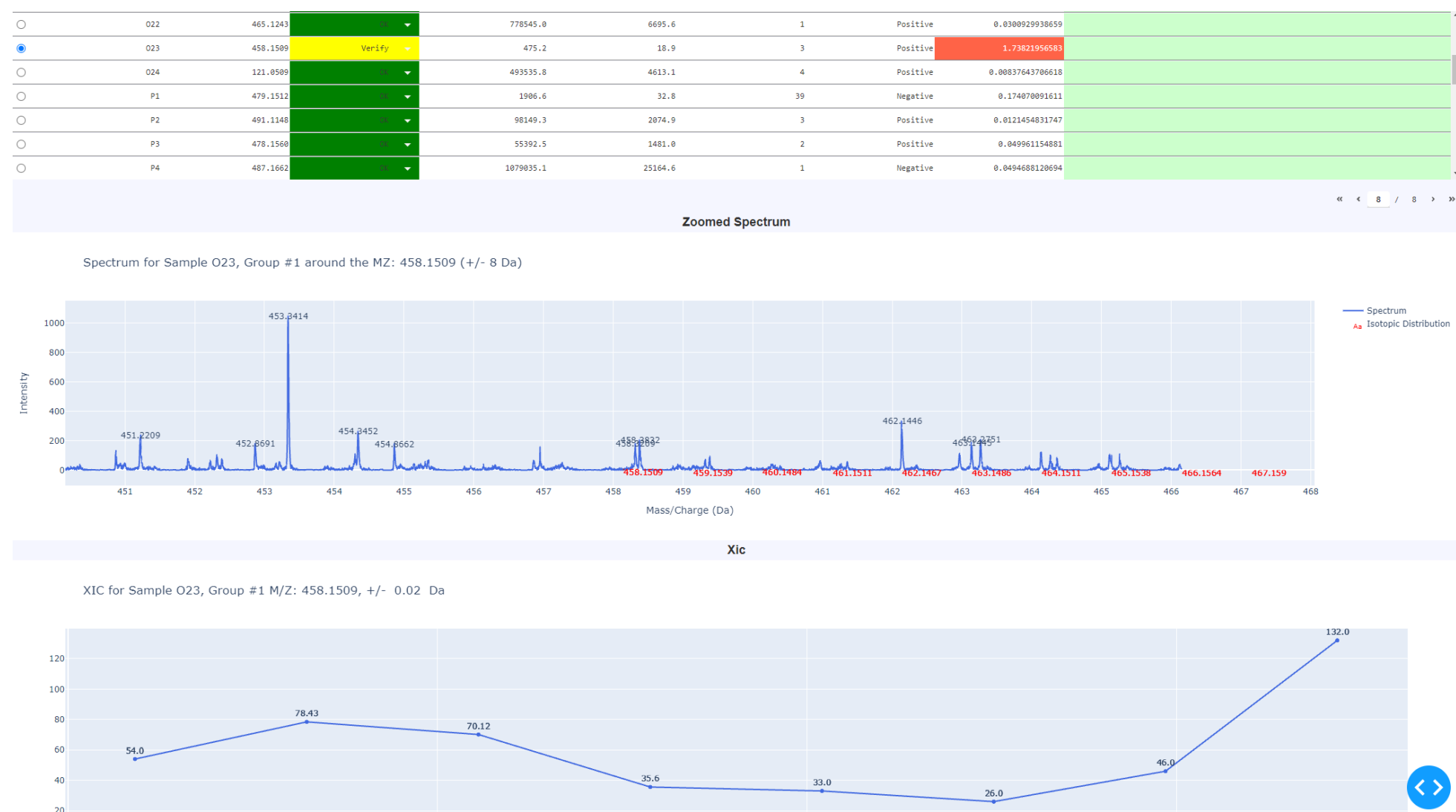
Figure 6. Example of a sample well (Q23) did not meet the validation rules, with its mass spectra and XIC directly visualized for review
