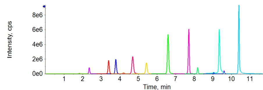
**Figure 1.** Overlaid extracted chromatograms (XIC) of 14 UV filters commonly found in commercial sunscreen in positive ion mode.
