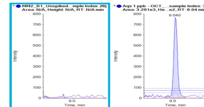
**Figure 2.** Detection of octocrylene in commercial sunscreen in comparison to octocrylene standard in solvent. (Left) Commercial sunscreen showing no peak at the expected retention time for octocrylene, confirming the label claim. (Right) An XIC of octocrylene standard at 1 ng/mL in solvent.
