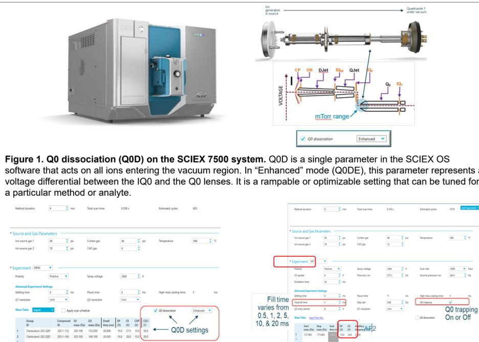
**Figure 1. Q0 dissociation (Q0D) on the SCIEX 7500 system.** Q0D is a single parameter in the SCIEX OS software that acts on all ions entering the vacuum region. In “Enhanced” mode (Q0DE), this parameter represents a voltage differential between the IQ0 and the Q0 lenses. It is a rampable or optimizable setting that can be tuned for a particular method or analyte.
