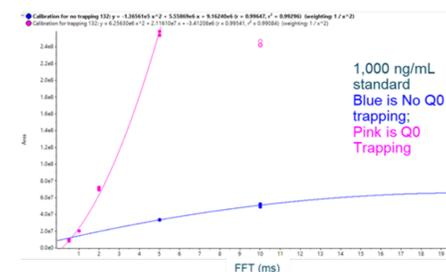
**Figure 4. Impact of FFT and Q0 trapping on signal for the LIT-MRM<sup>3</sup> workflow.** Increasing FFT increased the signal intensity for the MRM<sup>3</sup> data trace. Turning on Q0 trapping quickly saturated the detector and therefore limited the LDR. The same pattern was observed for both secondary product ions assessed.
