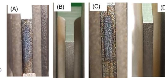
**Figure 8.** When the highly accelerated infusion test was conducted with the Q0 T-bars imposing a high m/z cut-off around m/z 850, the system was able to pass all tests with 204 mL of cannabis matrix infused. Very large build up of debris on one pair of T-bars (A,C) and this kept the Q1 cleaner for a longer period of time. As expected, the other pair of T-bars was clean (B,D). The Q0 T-bar mass window did not drift with up to 204 mL of matrix infusion.
