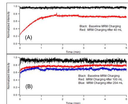
**The T-bars reduced contamination of Q1 and improved robustness by more than 5X.**
