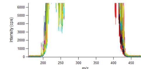
**Figure 5.** Overlay of Q1 windows transmitted in the 10 different overnight matrix infusions. Bandpass windows generated by T-bars did not shift when up to 100 mL of tea/arugula matrix was sprayed.
