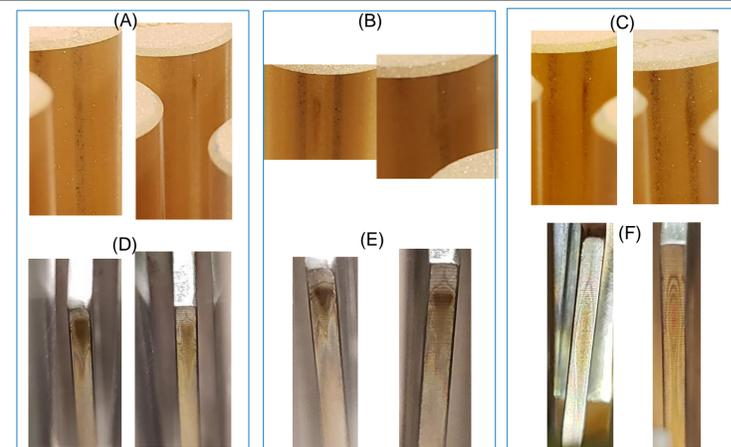
**Figure 4.** Clean Q1 rods observed after infusing 100 mL of tea/arugula matrix with (A) T-bars/Q0 transmitting m/z 200-400, (B) T-bar/Q0 transmitting m/z 400-800, and (C) T-bar/Q0 transmitting <m/z 900. The debris were observed on one pair of T-bar electrodes where filtered high-mass ions were deposited under three bandpass configurations respectively (D-F).
