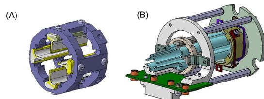
**Figure 1.** Illustrations of (A) T-bar assembly and (B) the assembly comprising T-bars on Q0 ion guide
