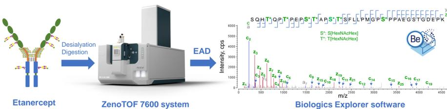
**Figure 1. Elucidation of O-linked glycosylation in etanercept using the ZenoTOF 7600 system and Biologics Explorer software from SCIEX.** EAD is powerful for the localization of labile glycosylation. The sites of glycosylation in the O-linked glycopeptides of etanercept that contained up to 7 O-linked glycan structures were confidently determined based on the interpretation and annotation of EAD MS/MS spectra using Biologics Explorer software.
