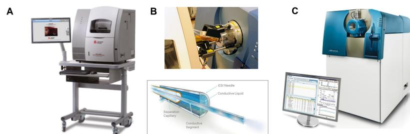
Figure 1. A. CESI 8000 Plus. B. CESI-MS interface. C. TripleTOF<sup>®</sup> 6600
