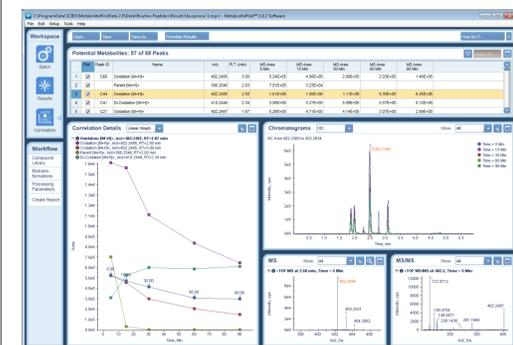
Figure 9. The correlation workspace of MetabolitePilot 2.0 software displaying results of the Buspirone incubation experiments. Shown on the correlation plot are the results for the parent compound, N-oxide, 6'-OH, 5,6'-di-OH and 3'-OH.
