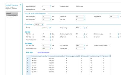
Figure 2. SCIEX OS SWATH method setup window for haloperidol. Seven variable SWATH windows were used to cover the expected Phase I biotransformations.
