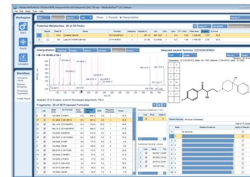
Figure 7. The interpretation workspace of MetabolitePilot 2.0 software displaying results of the top oxidized metabolite of haloperidol. MetabolitePilot assigned the site of hydroxylation to the alkyl chain.
