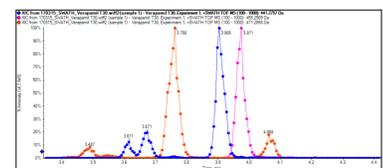
Figure 3. LC-MS chromatogram from the SWATH acquisition of a RLM sample of verapamil. The pink trace is the parent compound, red trace oxidized metabolites and blue trace is demethylated metabolites. The average peak width is ~5 seconds, and each peak has 10-12 points. The resolution of the demethylated parent was >37 000 and MS/MS was >30 000 for the characteristic 289.19 ion.
