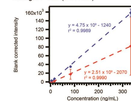
Figure 5: Calibration curves of fragile peptides in BSA digest. The signal improvement and noise reduction from the addition of ACN increases the sensitivity of a standard IDA method for the highest charge state of fragile peptides.
