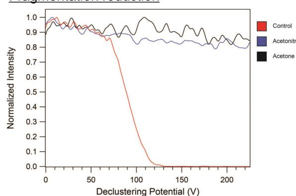
Figure 2: Normalized XIC of a declustering potential ramp of 4+ KGAIL. By ramping DP, fragmentation of the 4+ ion is induced resulting in loss of intensity with increasing DP.
