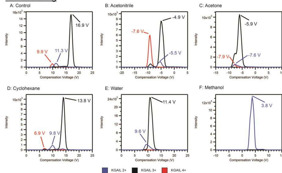
Figure 1: CoV ramps of KGAIL under different modifier conditions.
