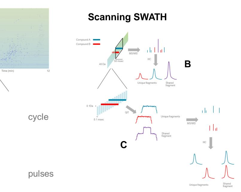
Scanning SWATH acquisition. During each cycle, the isolation window for MS/MS is sliding along the m/z range of interest. At each pulse, the isolation window is shifted slightly higher in m/z. The data from every pulse is
