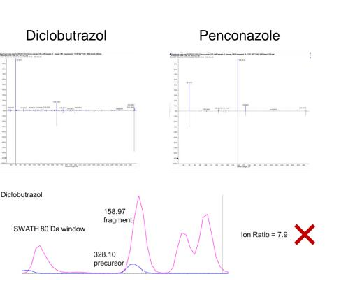
Diclobutrazol and penconazole almost perfectly coelute. These compounds have an identical fragment (158.97 Da). In traditional SWATH acquisition, both of these compounds were fragmented in the same SWATH acquisition window. This made it difficult to determine of one, the other, or both compounds were present
