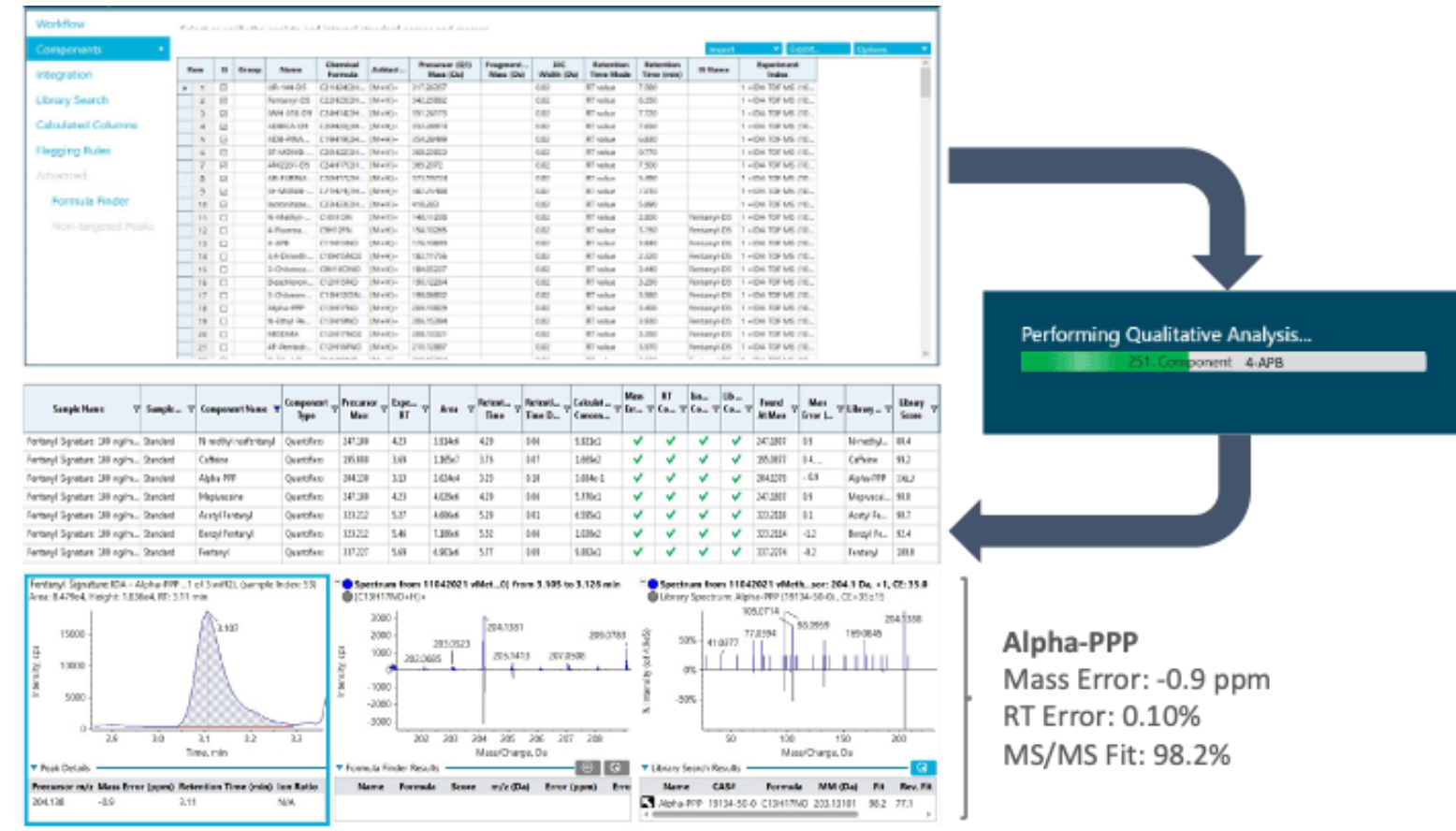
Figure 5. Retrospective analysis performed on a previously acquired dataset using SCIEX OS software. Data acquired using an authentic case sample was reprocessed after modifying the processing method window by adding the 130 NPS included in this panel (top). The stimulant Alpha-PPP was retrospectively identified in the authentic case sample from the SWATH DIA data. A precursor mass error of -0.9 ppm, retention time error of 0.10% and an MS/MS fit score of 98.2% provided excellent measures for the confident identification of Alpha-PPP in the postmortem case sample.
