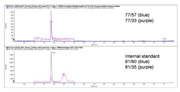
Figure 1. Example chromatogram of a 0.1 ng/mL standard of sodium fluoroacetate with internal standard
