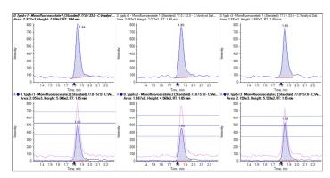
**Figure 2.** Repeat analysis at 0.1 ng/mL standard, 2 MRM transitions were monitored and the ratio of quantifier (top) and qualifier transition (bottom) was used for compound identification, 30% MRM tolerances are displayed in the peak review following SANCO/12571/2013)
