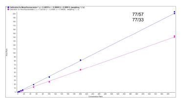
**Figure 3.** Calibration lines from 0.02 to 500 ng/mL for the quantifier ion (blue) and 0.05 to 500 for the qualifier ion (purple)
