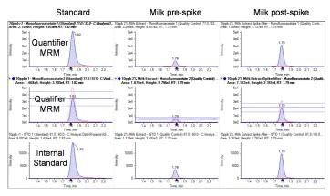
**Figure 4a.** Chromatograms of a standard in comparison to the preextraction and post-extraction spike of milk at 10 ng/mL; quantifier ion (top), qualifier ion with ratio tolerances (middle), and internal standard (bottom)
