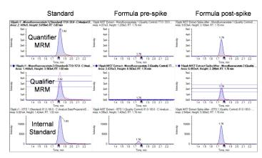
**Figure 4b.** Chromatograms of a standard in comparison to the pre-extraction and post-extraction spike of infant formula at 10 µg/kg; quantifier ion (top), qualifier ion with ratio tolerances (middle), and internal standard (bottom)
