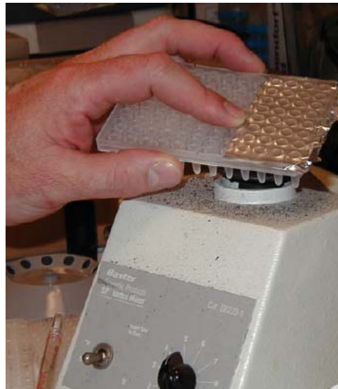
Figure 1. (Top) Sealing the reaction plate with aluminum foil. (Bottom) Vortexing the plate.
