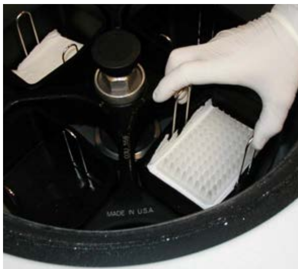
Figure 3. The inverted plate containing the folded paper towels is placed into the rotor.
