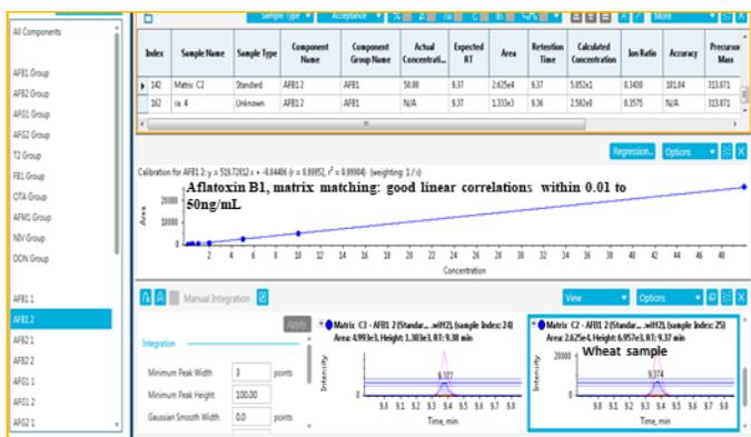
Fig 9. Quantification results for AFB1 in wheat as they appear in the SCIEX OS software user interface
