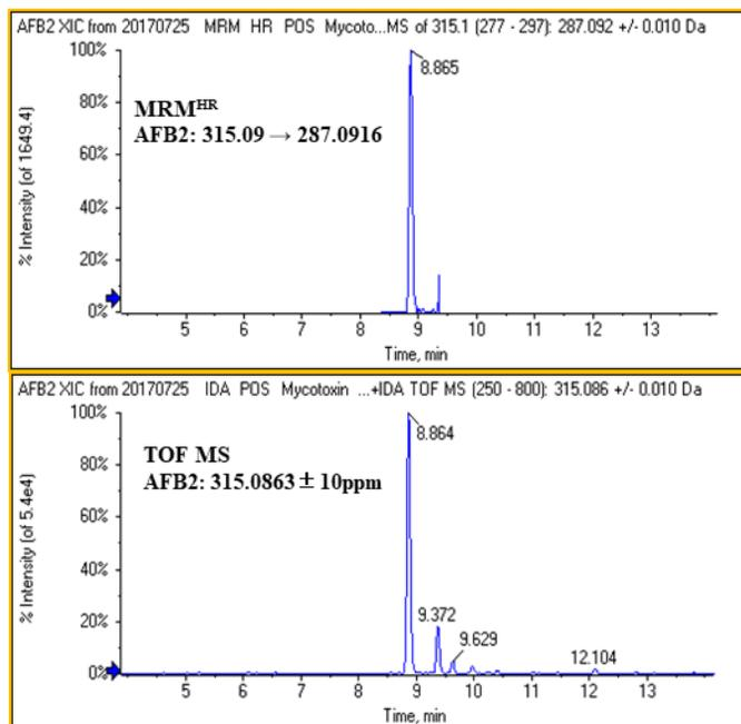
**Fig 6. Scheduled MRMHR selectivity for AFB2 compared to TOFMS; increased selectivity with MRMHR reduces the potential for false negatives or incorrect integration of different peaks.**
