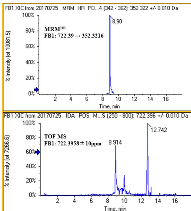
**Figure 1. Scheduled MRM<sup>HR</sup> selectivity compared to TOFMS for FB1.** Increased selectivity is demonstrated by monitoring the ion transition using MRM<sup>HR</sup> compared to monitoring solely the target precursor ion and reduces the potential for false negatives or incorrect integration of matrix peaks.
