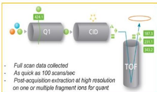
Figure 2. High Resolution MRM (MRM<sup>HR</sup>) ion path.
