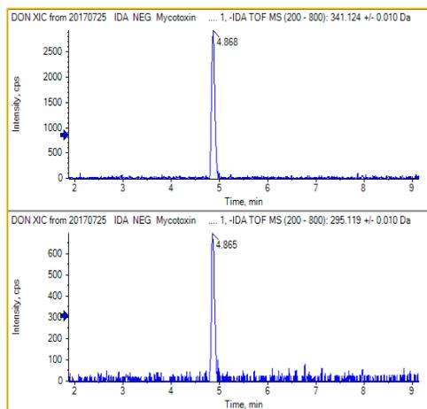
Fig 6. Chromatogram of DON: formate adduct (top) produced greater absolute signal than dehydrogenated precursor (bottom).
