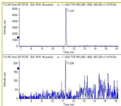
Fig 5. Chromatogram of T-2: ammonium adduct (top) produced a greater absolute signal versus protonated precursor (bottom).
