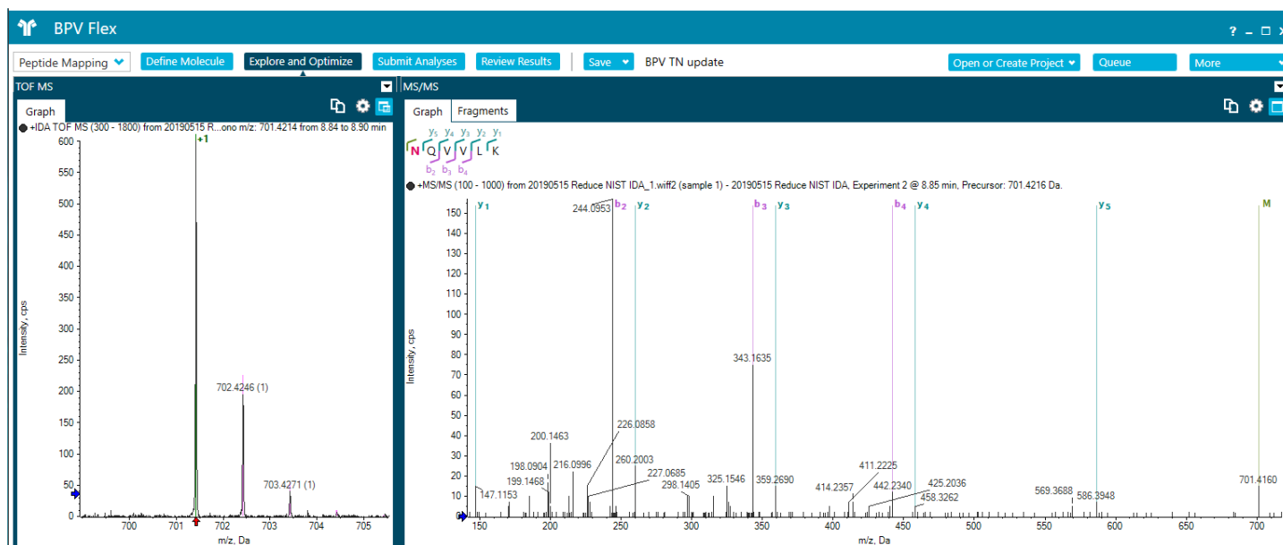
Figure 1. Review of MS and MS/MS deamidated NQVVLK peptide of NISTmAb in BPV Flex Software using customizable review interface. MS graph provides information on charge state and overlay with theoretical isotope ratio for increased confidence in the assignment. MS/MS pane shows fragment ions (b and y ions) and precursor (M) in addition to an overview of the MS/MS sequence coverage information.
