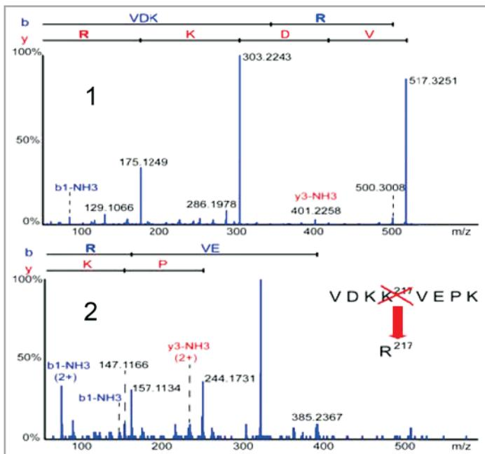
**Figure 3.** MS/MS spectra for trastuzumab (1) and trastuzumab-B (2), showing the absence of the fragmentation ions m/z 517.3095 (1+) for trastuzumab-B and the presence of m/z 314.6937 (2+) characterizing the amino acid substitution of lysine to arginine.
