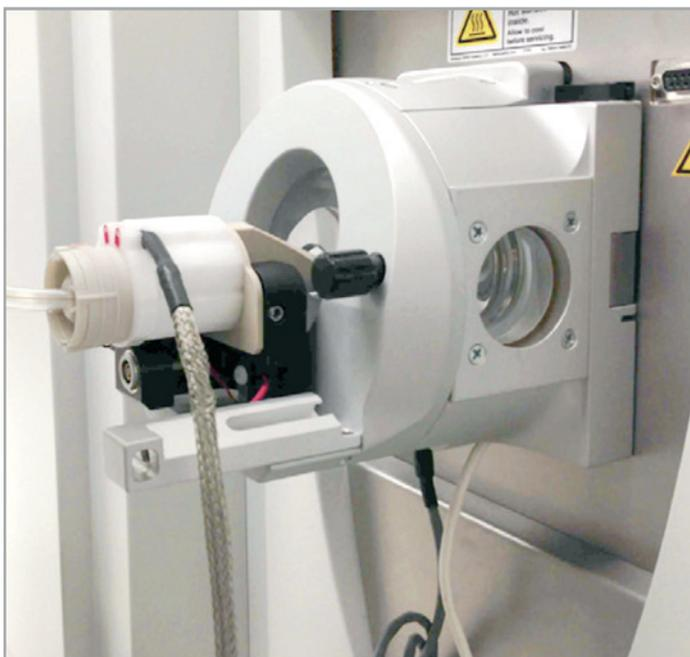
**Figure 1B.** The OptiMS sprayer connected to a Thermo Scientific Nanospray II ion source.
