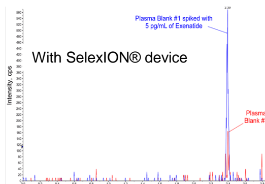
MRM chromatograms of plasma samples analyzed with and without SelexION ® device
