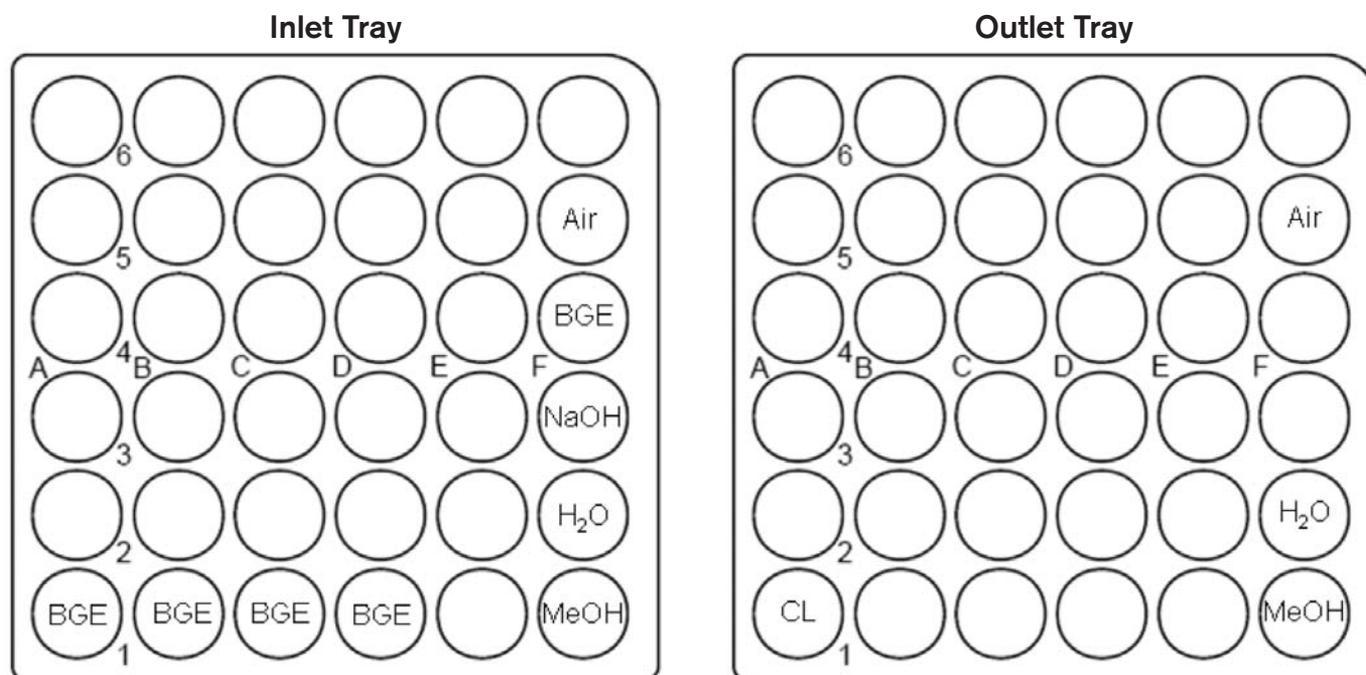
Figure 7: Buffer tray vial configuration for all methods.
