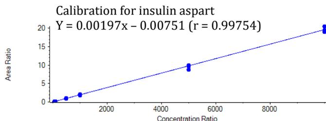
**Figure 4.** Calibration curve for quantitation of insulin aspart in human plasma (50 pg/mL to 10 000 pg/mL).
