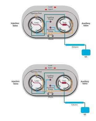
**Figure 1.** Valve positions for the trap loading part of the method (top) and the analysis part of the method (bottom).
