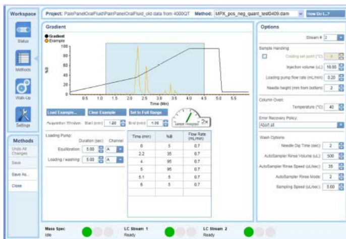
Figure 1. MPX chromatographic method. By applying MPX, the injection-to-injection time can be shortened to 3.5 min
