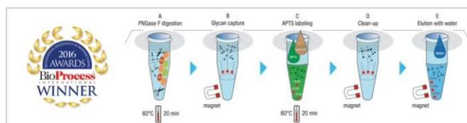
**Figure 4. The Fast Glycan Workflow.** (Top) Labeling and analysis kit – P/N B94499PTO. (Bottom) Fast Glycan Sample Preparation Workflow.
