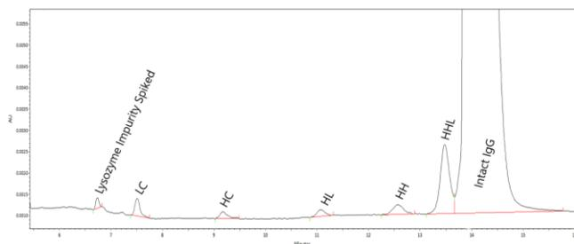
**Figure 8. Representative Electropherogram of NIST Antibody.** NIST under non-reducing conditions showing its low-level impurities, including the quantitation of 0.05 mg of lysozyme spiked into 1 mg of NIST antibody.
