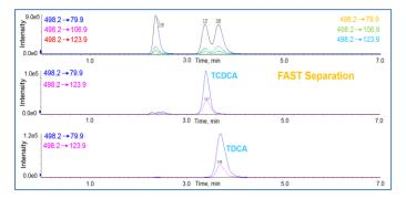
Fast Separation of Bile Acids with an Isocratic LC Method. Without SelexION Technology, the two isobaric bile acids TDCA and TCDCA cannot be completely separated from each other. Confident identification and accurate quantitation would be difficult due to the overlap of the two LC peaks. Separation of these isobaric bile acids is possible by SelexION technology using the specific compensation voltages for these compounds.
