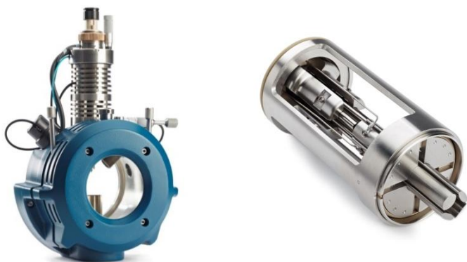
Figure 1. IonDrive ™ Turbo V Source and IonDrive ™ QJet Ion Guide. High efficiency heaters provide efficient desolvation and ion production for high sensitivity at high flow rates. Dual RF stages maximize ion sampling from a large orifice while increasing ion transfer efficiency into the Q0 region – without increasing vacuum load in the analyzer region.
