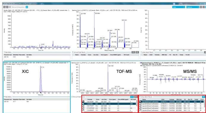
Figure 8a. Review of XIC of m/z 226.134 at RT 8.2 min and spectra with a found formula of C 14 H 15 N 3 , although ranked second based on mass accuracy the high ChemSpider hit count revealed the correct match
