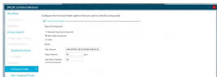
**Figure 5b.** Method editor in SCIEX OS software for unknown identification, configuration of formula finding options
