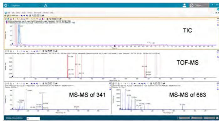
**Figure 3.** Simultaneous acquisition of TOF-MS and MS/MS using IDA, the example shows spectra of sucrose and sucrose dimer of the matrix
