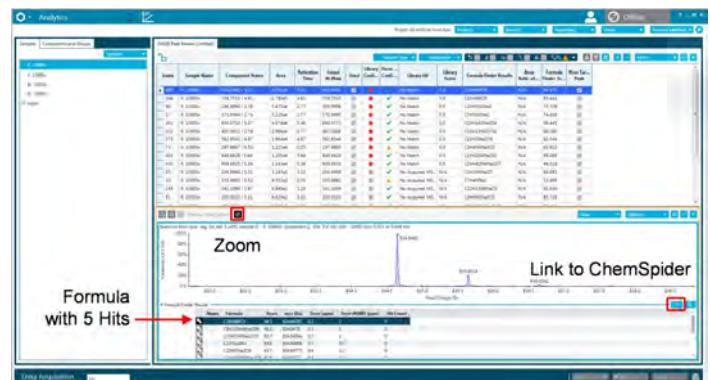
**Figure 7.** Zoom into TOF-MS to display detailed results of formula finding, the most likely formula has a mass error of 0.3 ppm in TOF-MS an average mass error of 1 ppm of all fragments in MS/MS and 5 matching structures in ChemSpider
