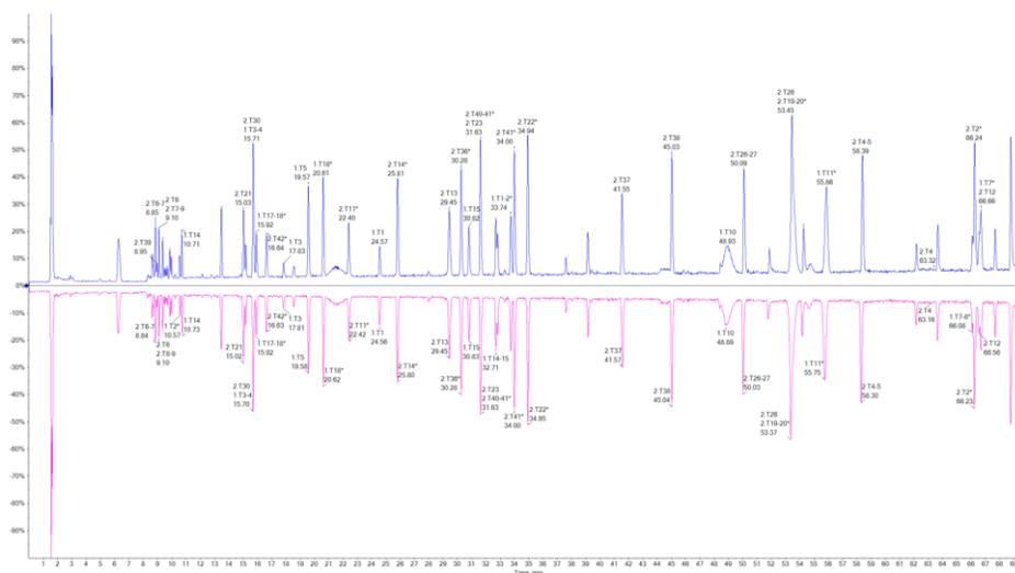
**Figure 1. Peptide Mapping LC Traces.** Mirror plot of standard (top) and test sample (bottom) peptide maps collected a SCIEX TripleTOF 6600 system and processed with BioPharmaView 2.1 software. Excellent agreement on retention time and peak identification observed between samples.
