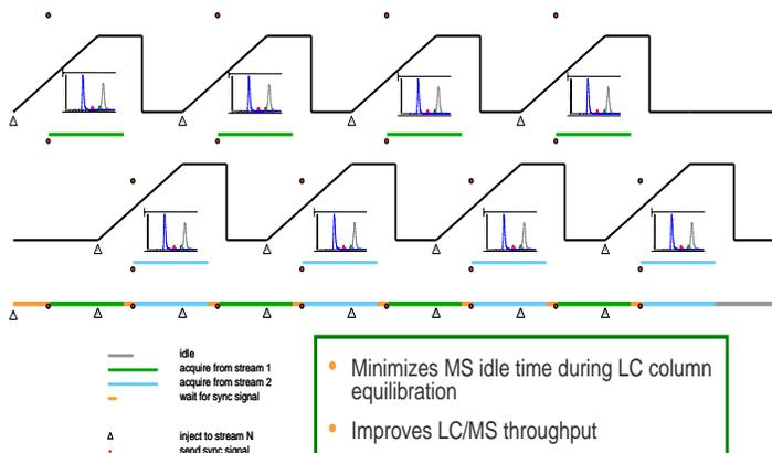
Figure 1. Multiplex LC system Designed to Support Two Parallel LC Streams into a Single MS
