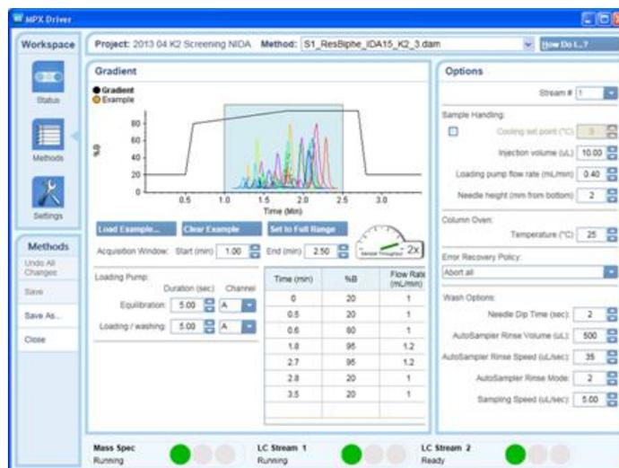
Figure 3. MPX® TF Driver 1.0 interface with exemplary LC configuration and method.
