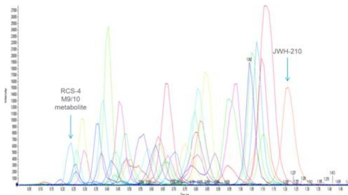
**Figure 5. Extracted ion chromatograms of all analytes that elute during a 1.5-min data window.**
