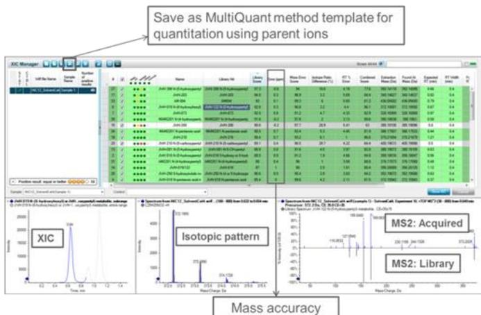
Figure 6. PeakView® software with MasterView™; the top pane shows an XIC table loaded for target drug screening and identification
