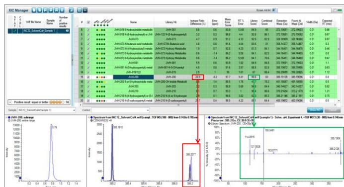
Figure 8. Interference caused isotopic ratio change, but MS/MS confirmed identity and eliminated possible false negative caused by elevated isotope ratio difference for JWH-200 in neat solution.
