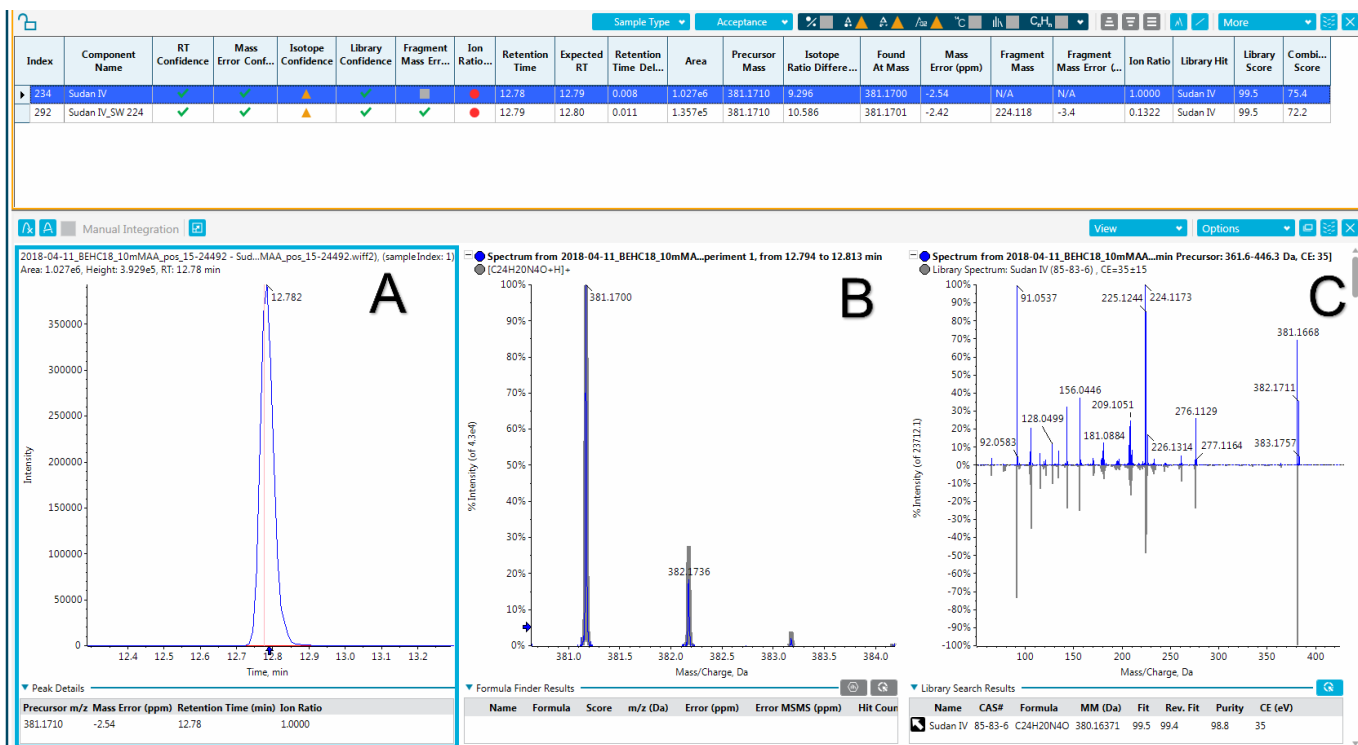
Figure 5: Qualitative Results for a Sample Contaminated by Sudan IV. A) Chromatographic peak showing precursor and retention time. B) High resolution MS data including matching the observed isotope pattern to that of the target analyte. C) Matching of the MS/MS spectrum collected by SWATH acquisition to that of the target analyte in the spectral database.
