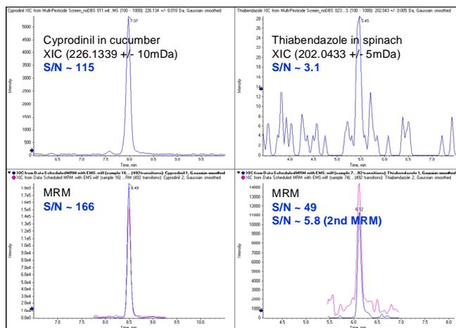
**Figure 3.** Comparison of Signal-to-Noise (S/N) of pesticides detected in fruit extracts using the AB SCIEX TripleTOF™ 5600 System in TOF-MS mode (100ms accumulation time) vs. the QTRAP® 5500 System using Scheduled MRM™; the difference in S/N depends of the fragmentation efficiency of the detected analyte
