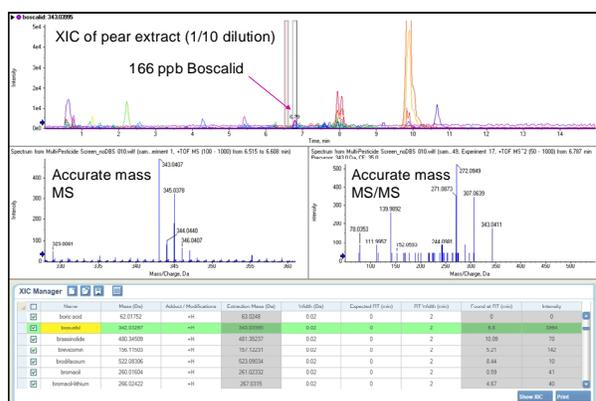
**Figure 6:** The pesticides Boscalid (Pyraclostrobin, Spinosyn A and D, and Trifloxystrobin spectra not shown) were identified and quantified using accurate mass MS and MS/MS information in a pear extract using the XIC Manager of PeakView™ Software
