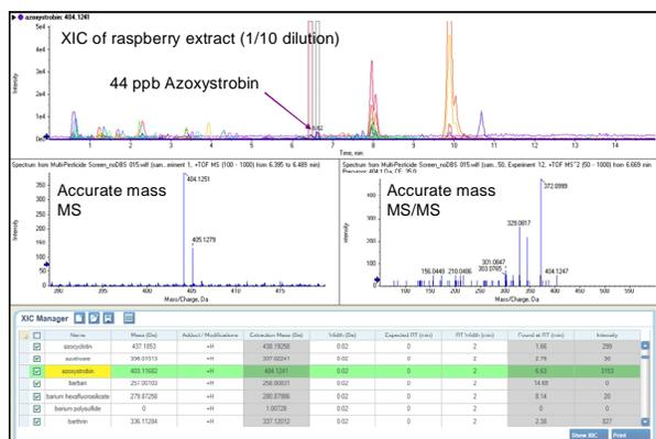
**Figure 4:** The pesticides Azoxystrobin (and Cyprodinil, spectra not shown) were identified and quantified using accurate mass MS and MS/MS information in a raspberry extract using the XIC Manager of PeakView™ Software
