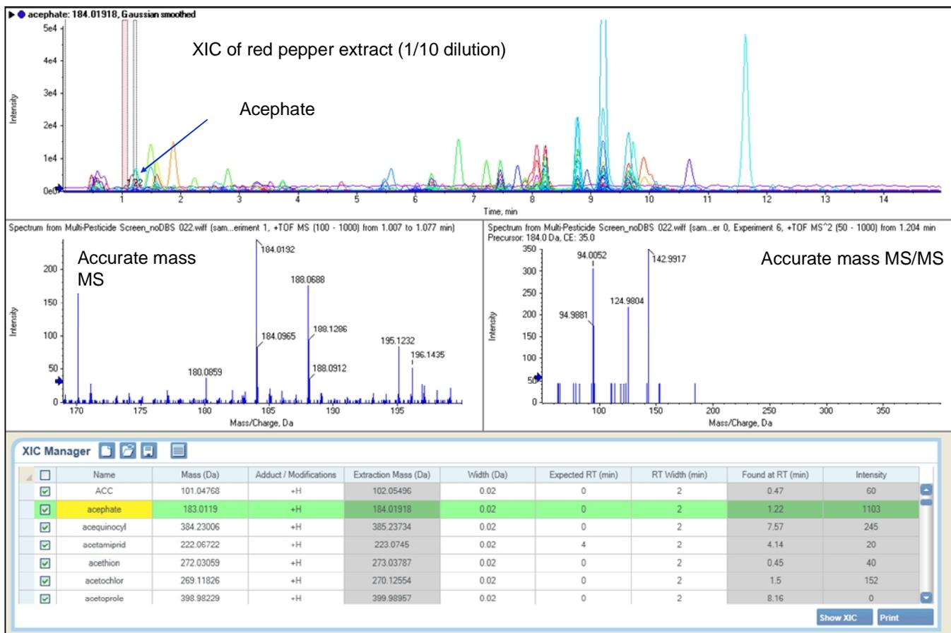
**Figure 6:** The pesticide Acephate was retrospectively confirmed in an extract of red bell pepper after previous GCxGC-TOFMS screening based on accurate mass MS and MS/MS information
