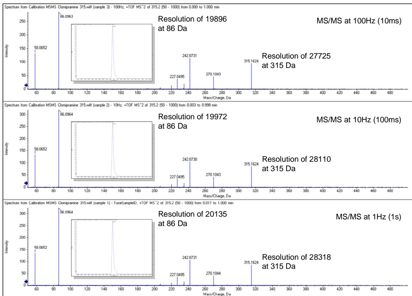
Figure 1. Highest resolution at every scan speed over the entire mass range with stable mass accuracy of  $\sim$ 1 ppm
