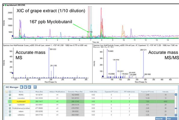
**Figure 5:** The pesticides Myclobutanil (Iprodion, Pyrimethanil, and Spinosyn A and D, spectra not shown) were identified and quantified using accurate mass MS and MS/MS information in a grape extract using the XIC Manager of PeakView™ Software
