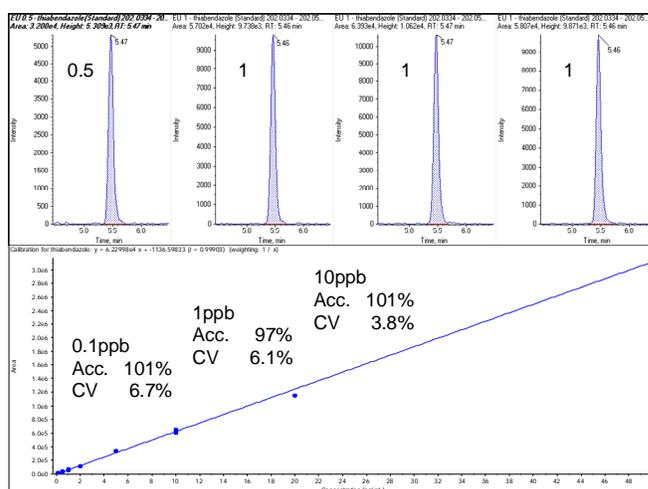
**Figure 2.** Calibration lines (0.05 to 50ppb) and statistical results (triplicates) at different concentrations for the two selected pesticides Cyprodinil and Thiabendazole
