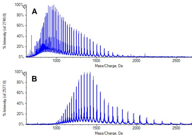
Figure 3: Raw MS spectrum of denatured and completely reduced NIST mAb heavy chain (A). Raw MS spectrum of selectively reduced NIST mAb heavy chain (B).
