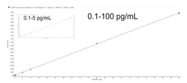
Figure 3. Linear Calibration Curve. The linear calibration curve was found to be linear from 0.1 - 100 pg/mL for testosterone in neat solvent, using SelexION+ Device.
