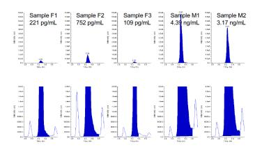
**Figure 5. Example Data in Matrix.** Example data of testosterone analysis in serum is shown, showing zoom on y-axis, to visualize separation of interferences and low chemical background due to the use of the ion mobility filter.
