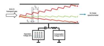
Figure 1. SelexION+ Differential Mobility Separation Technology. This device consists of two planar electrodes. Voltages are applied, which serve to filter out isobaric interferences prior to detection by tandem mass spectrometry.
