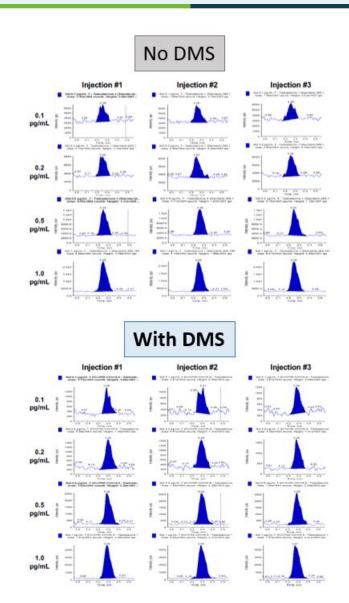
Figure 4. Evaluation of Detection Limits. Comparison of LOQ and S/N, in neat solvent, with and without the SelexION+ Device.
