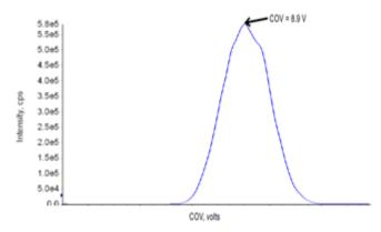
Figure 2. Optimization of COV Parameters for Testosterone.
