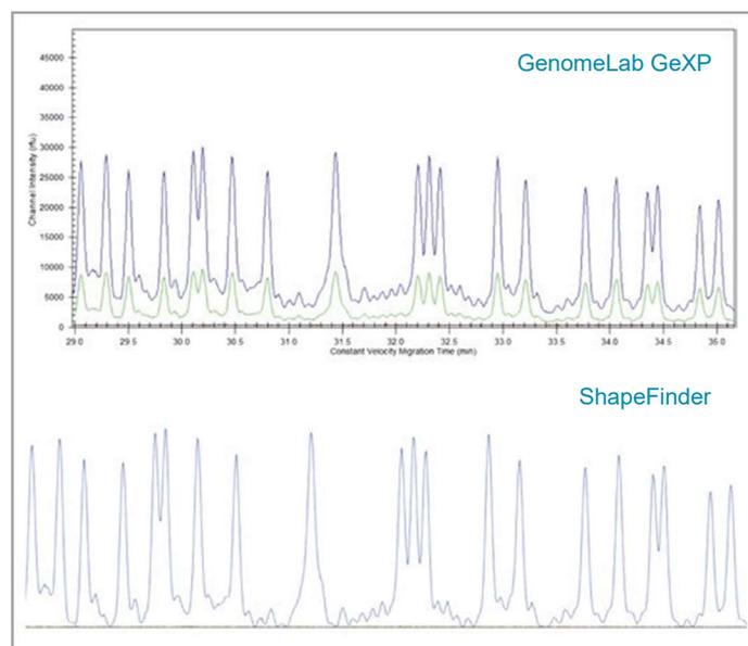
**Figure 4a.** GenomeLab GeXP raw electropherogram (zoomed image) showing IDT Cy5 Dye (blue trace) cross-talk to another channel (green trace). Bottom image shows ShapeFinder cross-talk correction by applying Matrixing-2.1.
