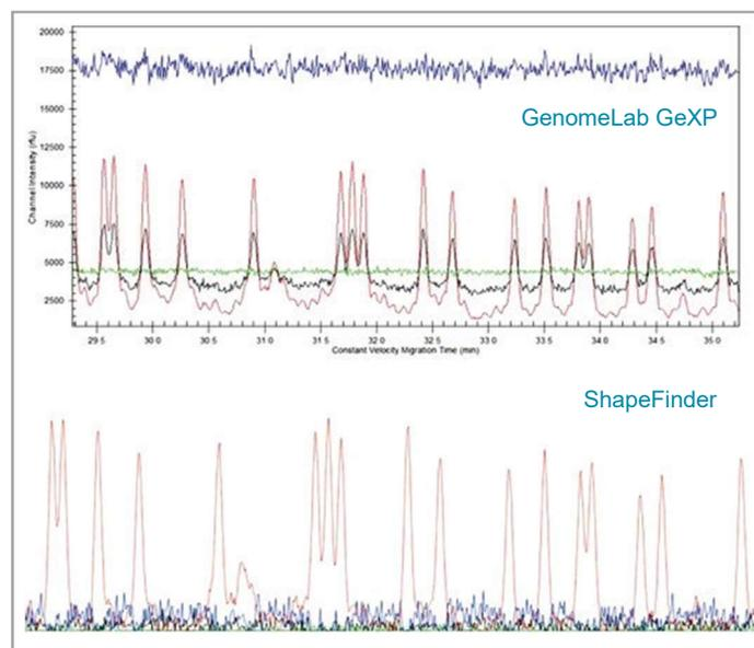
**Figure 4b.** GenomeLab GeXP raw electropherogram (zoomed image) showing IDT LI-COR IRDye 800CW Dye (red trace) cross-talk to another channel (black trace). Bottom image shows ShapeFinder cross-talk correction by applying Matrixing-2.1.
