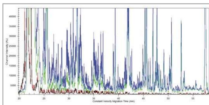
**Figure 5.** Raw superimposed electropherograms show SHAPE positive (Cy5, blue trace) and negative (Cy5.5, green trace) reactions, and sequencing ladder reactions: ddATP (Alexa Fluor Dye 750, black trace) and ddTTP (IRDye 800CW, red trace), for the HPRT1 RNA transcript fragment up to the first 408 bases.
