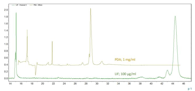
**Figure 1.** Overlaid electropherograms of the analysis of a monoclonal antibody using the standard CE-SDS analysis method with UV detection (5kv, 20s), and an optimized CE-SDS analysis using LIF detection (2.5 psi, 10 s injection).
