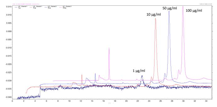
Figure 7. The effect of varying the sample concentration on peak resolution. Each sample (2.5 psi, 5 s injection) was analyzed using the same separation conditions (13 kV, effective separation length 20 cm, 40 °C).
