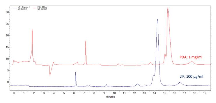
Figure 2. Red trace is the analysis of IgG (1 mg/mL) by CE-SDS using UV detection (PDA detector) offset by 1 minute. Blue trace is the analysis of IgG (0.1 mg/mL) by CE-SDS using LIF detection. In this example both samples were injected electrokinetically (5kV, 20 s)
