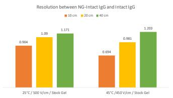
**Figure 5**. The impact of effective length and temperature on the separation and resolution of the NG species for the IgG parent peak using the same injection conditions.
