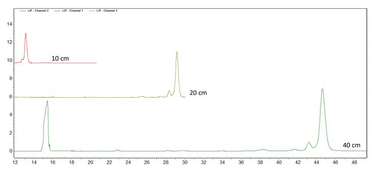
Figure 4. Comparison of an injection of 100 µg/mL IgG standard using LIF detection and different capillary lengths. Each sample was injected at 5kV, for 20 s at 45 °C, with an effective field of 450V/cm.
