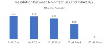
**Figure 6**. The effect of the injection amount on the resolution between NG and IgG peaks. All separations were performed at 13 kV, 40  $^{\circ}$ C using an effective capillary length of 20 cm using a 100 µg/mL sample.
