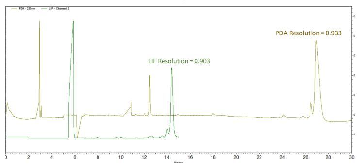
Figure 8. Comparison of optimized classical PDA UV method (20 cm effective separation length, brown trace) with optimized short LIF method (10 cm effective separation length green trace).
