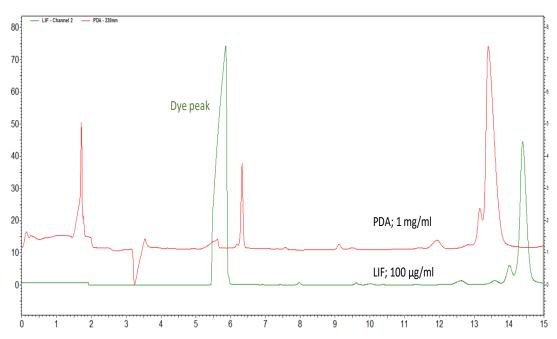
Figure 3. Comparison of an injection of an IgG using LIF detection (green trace, 13.5kV, 40 °C) versus PDA detection (Red trace, 15kV, 25 °C) using an effective separation length of 10 cm and the same injection conditions.
