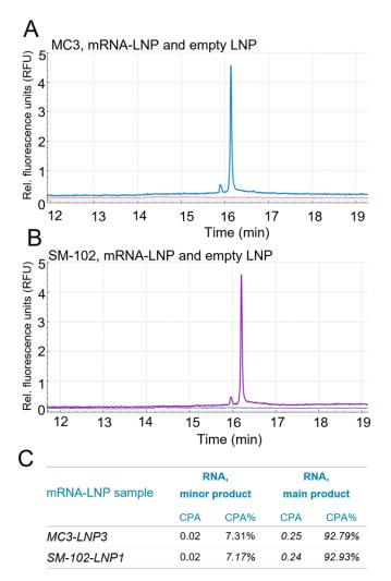
Figure 7. Nucleic acid content profiling from mRNA-LNP formulations with distinct ionizable lipids. (A) MC3 and (B) SM-102 mRNA-LNP formulations with a similar amount of mRNA starting material were evaluated for nucleic acid content by CGE-LIF. (C) Table illustrating the CPA and CPA% values for the minor and main products observed in these 2 formulations.
