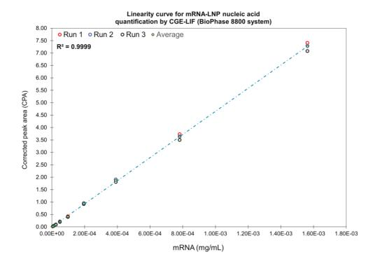
Figure 9. Linearity of mRNA for nucleic acid analysis. The CPA of the main RNA product was used to construct a linearity curve across 9 mRNA concentrations. The regression analysis was performed on the average of 3 injections. The  $R^2$  value for the linear regression analysis was 0.9999. The LLOD was 6.10 x 10<sup>-6</sup> mg/mL, the LLOQ was 1.22 x 10<sup>-5</sup> mg/mL and the ULOD was 1.56 x 10<sup>-3</sup> mg/mL.
