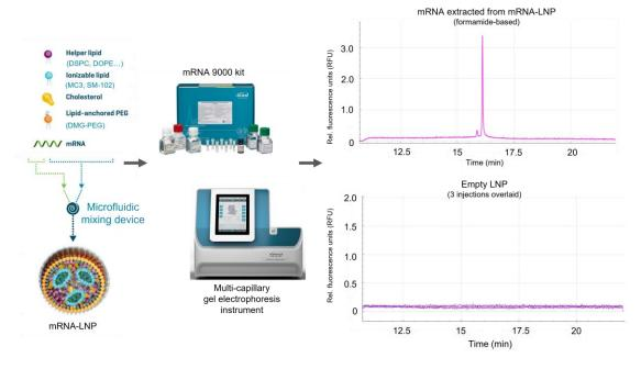
Figure 1. Simplified workflow to assess nucleic acid integrity of mRNA-LNPs with the multi-capillary BioPhase 8800 system and the RNA 9000 Purity & Integrity Analysis kit. The top panel shows a representative profile of RNA extracted from an MC3-based mRNA-LNP product. The bottom panel shows the overlay of 3 empty MC3-LNP products. p 1
