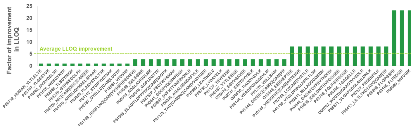
Figure 1. Factor of improvement in LLOQ for peptide quantification with Zeno MRM HR compared to MRM HR . On average, a 5-fold improvement in LLOQ for peptide quantification was observed with Zeno MRM HR in comparison to standard MRM HR .
